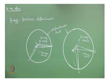
So, what I have drawn here is 2 types of 2 theta angle how this Bragg Brentano geometry or I would say Bragg Brentano far focussing method which is being adopted in this particular diffractometer. So, you have this is a diffractometer circle or goniometer circle
