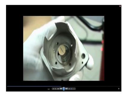
Now it is opened up this is your anode material it could be you can change this target material based upon the specimen you are analysing it could be a chromium or you know chromium target copper target and so on depending upon the type of sample you analyse and what the dismantle part is this is a close up view of this anode just for your information and this is that beryllium.
