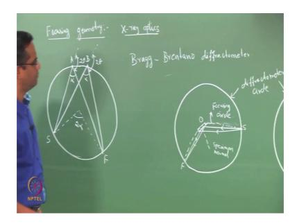
So, I will draw a focussing geometry. So, what I have drawn is a focussing geometry for X-ray optics suppose if you have the source here and then it goes to the sample and get
