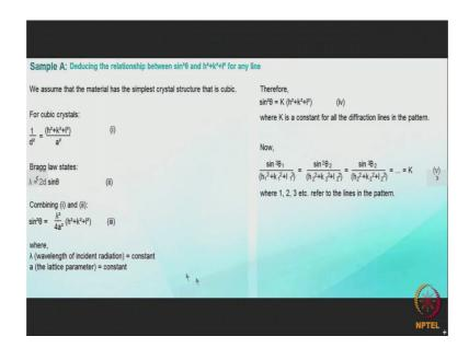
And the h k l values of that plane can be stated as 1 upon d square is equal to h square plus k square plus l square divided by a square where a is a lattice parameter of the material.
