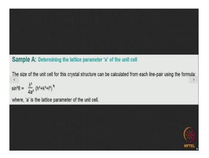
Now comes the third part of the problem; how to determine the lattice parameter of the unit cell? The material on the investigation now this can be done from this relationship which we found out earlier that for any line sin square theta is equal to lambda square by 4 S square into h square plus k square plus l square. So, we have now for every line found out the value of h square plus k square plus l square and the corresponding sin
