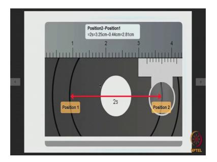
Say for example: this is my line pair 1 1. So, this is the position 1 for this line pair, this is the position 2 of the line pair. We find out with the help of the scale and the vernier what are the values here and what are the values there, and then we subtract one from the other. So, in this way we find out that this value 2 S for this line pair is simply equal to 2.81 centimetre c m.
