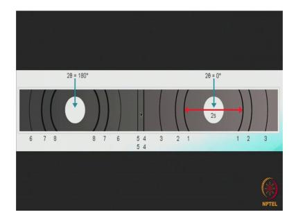
Say for example: this is an XRD pattern of an unknown substance. Now to begin with we assume the simplest possible crystal system for this material which is cubic. So, we assume the material has a cubic crystal structure. Now the first thing to do is to determine the distance between each of the line pairs which appear on the diffraction pattern.
