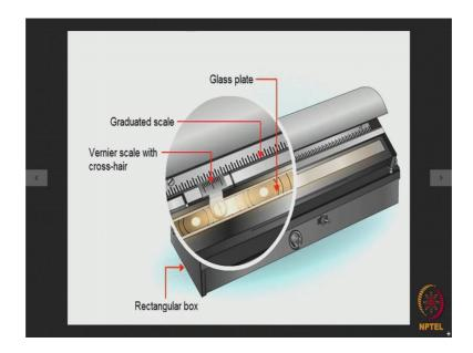
So, this we do using a rectangular box of this type which has got a glass plate here below which there is a source of light so that all the lines all the patterns are shown very clearly. There is a graduated scale along with a vernier in order to measure the line positions very very accurately.
