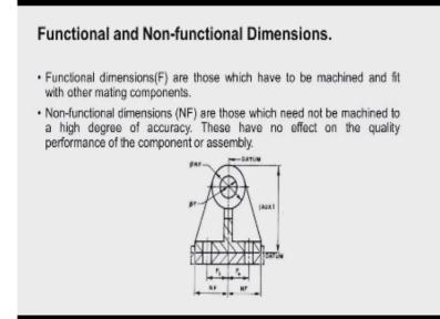
Now we should understand that when the dimensions of specified there are some functional dimensions and nonfunctional dimensions. If you see this diagram there are some dimensions like NF or non functional dimensions I can see if this is the outer surface of this particular third part where in NM will come in contact this place. So at this place when we not have to specify very stringent tolerance open tolerance will be alright.
