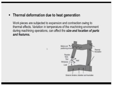
And then we have thermal deformation due to heat generation, now these work pieces there subjected to expansion and contraction or due to heat that is generated during manufacturing process, because variation in temperature this will be subjected it may to expand because the high the higher temperature. Now we can take example of work piece and then some milling operation is performed on the surface.
