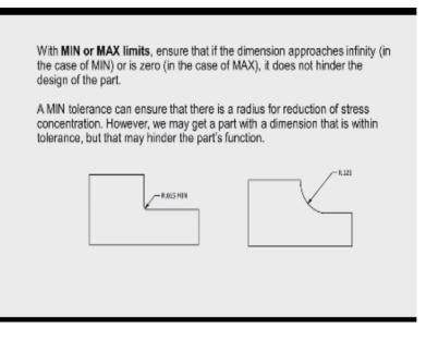
So such things one should consider and sometimes the minimum or maximum limit specified drawings we can see here we have a work part like this we have a flat here and the radius of the reflect 0, 0.015 minimum, now if we follow this the operator may produce a part with a radius of 0.125 millimetre. As per the specification this work this size is alone but whether it affects the functionality that we should consider.
