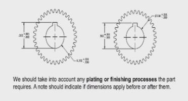
Now another important points to be considered a specified is the whether the tolerance is specified on radius or diameter. Now in this picture we can see the tolerance is provided on the radius, so 250+/- +0 001mm-0. Now in this diagram the tolerance is provided on the diameter that is 500+0.001 mm and the lower limit is 500 mm. So depending upon whether it is placed on radius or diameter the diameter will be vary.
