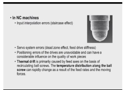
Now in case of NC machine the input interpolation error will be there because of that there will be staircase effect on the work piece like this, if we observe this picture here we can see there is some status effect ok, so now other reasons for dimensional changes is system errors like the dead zone effect and feed driver stiffness positioning errors of the drives and then that thermal drift is primarily caused by feed axes on the basis of re-circulating ball screw.
