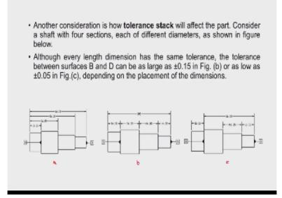
Now another consideration while allowing the as tolerance case, the tolerance stack now with a design engineer should understand what is the effect of this tolerance stack, we can see here we have three pictures wherein we have 4 circular features are there with varying diameter and they have the varying lens with some tolerances. Now if the tolerance is specified like this as shown in this diagram ok.
