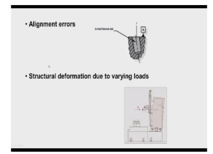
Now this is the error due to alignment error access cutting tool is not perpendicular to the surface because of that piece cutting forces acting on the structure the column of the machine tool because of that the column may deflect, so due to this also this work pieces size variation will occur.
