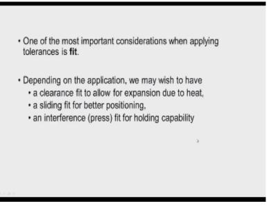
Now one of the most important consideration when applying tolerance is the fit, what is a kind of fit, I give the example of the bush shaft and the body, so between body and bush no
