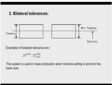
Now the second type of tolerancing is bilateral tolerance where in we have this basic size and tolerances is tolerance is provided on both side with the basic, so some example we can see here 25 is a basic size and the upper limit of the shaft is 25.02 mm and lower limit of the shaft is 24.98. Now the basic size is in between these two and deviation is allowed basic size is 25 millimeter, so the deviation is allowed on both sides of the basic size.
