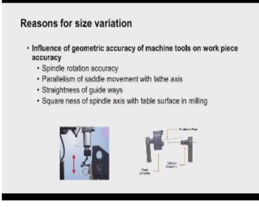
Now there are there are some of the reasons why the tolerances are specified and we will discuss about some of these points in detail, now the influence of geometric accuracy of machine tools on work piece accuracy, the manufacturer can see this picture here the machine tool will have some inherent inaccuracy like the movement of the spindle,. It may not be perpendicular to the table .
