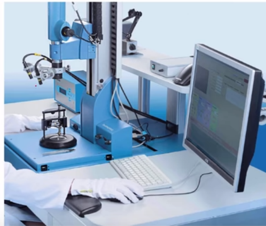
Alignment duration about 4 seconds Centering accuracy: 2 \mu\text{m}
