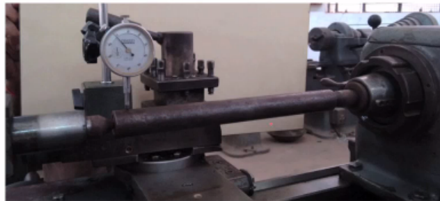
Alignment of both the centers in vertical plane
