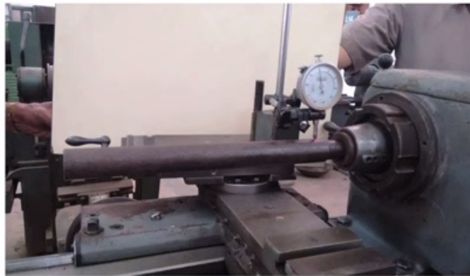
Measurement in vertical plane, free end upwards
