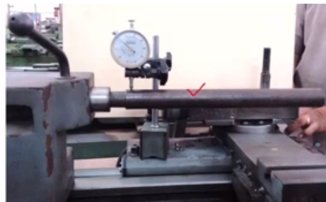
Parallelism of tailstock sleeve taper bore to the saddle movement – Vertical plane
