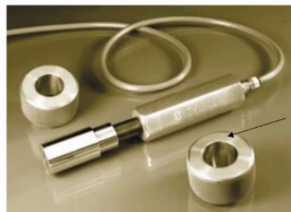
Master Two-nozzle air plug, with masters, for measuring inside diameter
