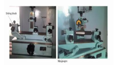
Now you can see and advance the sine center this is the base and then this is the sine table so it is pivot here okay. So this sign table can be tilted in this fashion. We can tilt the table and we can place here there is a roller and this is a surface design table, so here after lifting it after tilting it we have to fill this gap using the slip gauges.
