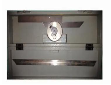
Now this picture shows the full set we have the body clamp peeping holes and then sliding blade with the 60 degree bevel on one side and 45 degree bevel on the other side and this is the blade which is fixed to the body and blade, which is slide. There is a spare a longer blade is provided so wherever necessary we can remove this smaller removal blade and we can insert this blade and we can use it.
