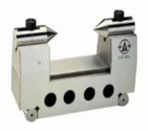
Now another variation of sign bar is a sine center you can see here we have the body of the sign Center these are the relief holes and then we have cylinders fixed to the body of the Science Center and then here we have 2 centers these the center they are slidable you can see the slot here we can loosen the clamp and then we can move the centers axially like this to accommodate the work piece of a different length.
