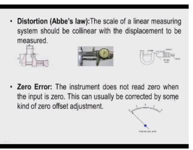
Now distortion is also known as Abbe's law. The scale of a linear measuring system should be collinear with the displacement to be measured. If you take the example of this vernier caliper we can understand that we keep the work piece between angle and spindle. So the axis of the work piece will be here, it is collinear with access the instrument. So in that case the distortion will be minimum.
