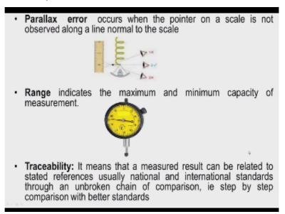
Parallax error this occurs when the pointer in a scale is not observed along a normal a line normal to the scale. Now this can understand with help of this diagram, we have the scale here, and we have pointer here, and the observer is observing the pointer from 3 different positions. This is position number 1, position number 2 and we have position number 3. When the observer observes the scale and pointer from the location 2 is observing the scale normally, then we get the correct real.
