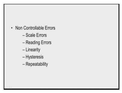
Now under non controllable errors these are these cannot be controlled but we can always measure what is the amount of error and then we can while repairing the inspection reports we have to account for these non controllable error you should know and accordingly we should represent the inspection reports.
