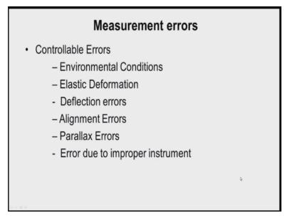
Now the measurement errors can be classified into controllable errors and non-controllable errors, under controllable errors means we can control the amount of these errors by adjusting the working environment. That means under controllable errors errors are due to environmental conditions, errors are due to elastic deformation, deflection errors, alignment errors, parallax errors and error due to improper instrument.
