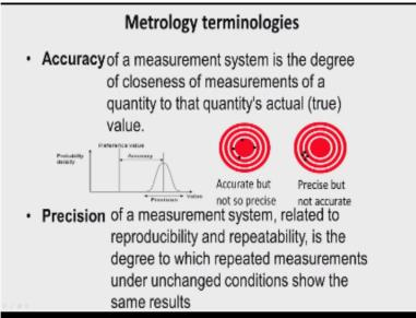
A first one is accuracy of the measurement system, it is the degree of closeness of measurements of a quantity to that quantities actual or true value. So we can understand the
