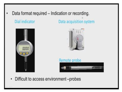
Now what is the data format that is required indication or recording, accordingly better if indication is required we should select the instruments with indications like the dial indicator with digital display and if recording is rich for recording of data is required then get a select data acquisition system having necessary or data acquisition speed, and data acquisition capacity.
