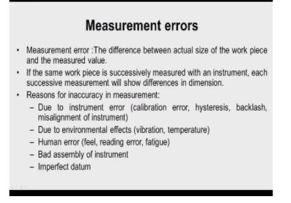
Now let us move to the next topic measurement errors, measurement error is the difference between the actual size of the work piece and the measure value. If the same work piece is successfully measured with an instrument each successive measurement will show differences in dimension, now what are the reasons for this, reasons for in accuracy in measurement are listed below.
