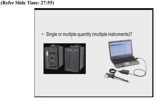
Then whether single or multiple quantity, how many instruments at a time we need to use, if we want 2, 3 or 4 or more than 2 instruments are there which are taking measurements then after data acquisition systems we should select accordingly which are having multiple channels or divisions. Sometimes we may have to dump the data measurement data to the soft ways data management soft ways for getting the statistical characteristics.
