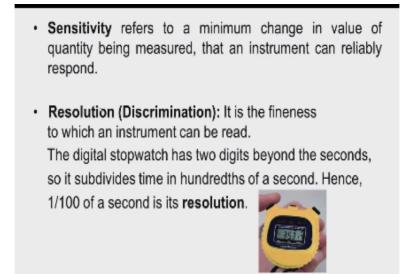
Now the second term is sensitivity of an instrument. This refers to a minimum change in value of quantity being measured that an instrument can respond. If I take an example of a dial indicator when we apply the displacement of point 1 millimeter and if the dial indicator is response to that signal, then we say the sensitivity of the dial indicator is 0.1 millimeter. And we have another term resolution, sometime it is also know as discrimination.
