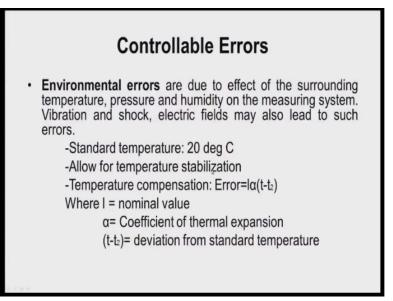
Now under controllable errors the first one is environmental errors, these are due to the effect of surrounding temperature variation the surrounding temperature, pressure and humidity or may be due to vibration and shock electric fields ok. Now we need to understand that when we conduct the measurement process we have to maintain a standard room temperature of 20 degree Celsius which is internationally accepted.
