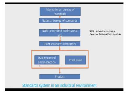
Now this is the manufacturing area where in the production is going on components are produced, assembled and then finally we get the product. During the process of production the quality control department will inspect all the components produced, but due to continuous usage of these instruments the instruments are subjected to be weir and the measurement here we seen.
