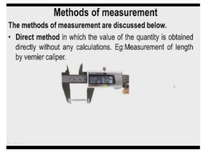
Now the next topic is methods of measurement, different kinds of measurement methods are used and we will discuss a few methods which are relevant to the metrology subject. The first one is direct method. In this method the physical quantity is of time directly without any calculation, example measurement of length by Vernier caliper. You can see that we have the component whose dimension, whose length is to be measured.
