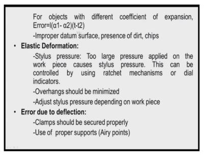
Now if you have two different kinds of material then the error can be calculated using this relationship, ltimes alpha-alpha2 times2-t-t2 where alpha 1 is coefficient of thermal expansion of the first material and alpha2 is coefficient expansion for second material. So measurement error maybe also due to improper datum surface which we discussed already and maybe there is presence of dirt and presence of chips.
