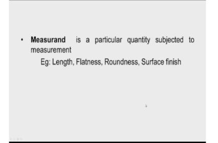
Now data measurement it is a particular quantity subjected to measurement, for example length, flatness, roundness, surface finish etc. These are measured quantities or measurement.
