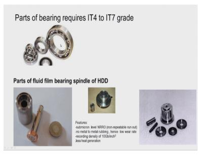
Now I am showing cube engineering parts, the bearings which require very fine finishes and very tight tolerances. We can see here we have some bearings, ball bearings with very fine finish. So, it is very essential that we have to control the dimensions. And it also necessary that we have to control the features, geometric features . For example the roundness or flatness, straightness etc., etc.
