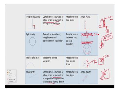
Now we will move to the perpendicularity or sometimes it is necessary that the two lines or two axis or two surfaces should be perpendicular to each other okay. There will be a datum surface and then there will be working surface. So, that angle between this working surface and this datum surface should be 90 degree. So that is known as perpendicularity, now how it i specify, they say we have an angle plate lie in this.
