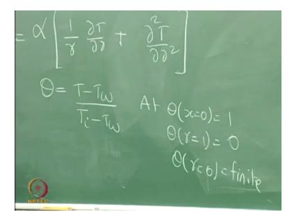
And  $\sigma$  at R = 1 will be 0 that will be t1 which is a constant so you need two boundary conditions with respect to radial direction so what is the other boundary condition should be finite or D  $\sigma$  by dr should be 0 okay so substituting this we can rewrite this as I can say my u = u m which is a constant based.
