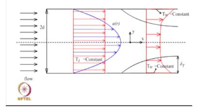
You so this is your assumption that at the inlet everywhere Inlet where you start the growth of the thermal boundary layer your Inlet temperature is uniform it is constant and so this is for the case if at X = 0 so now your coordinate starts from a point where you start the thermal boundary
