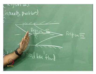
He Calls it as a rod-like flow so he assumes as it is like a solid rod which is passing through a circular tube okay so where do you have a velocity which is a constant and properties are also constant and at the starting point where you where you are looking at the thermal boundary layer okay so there the inlet temperature is a constant so the region that you are looking at now is where your velocity boundary layer smirched and then you start the thermal problem okay.
