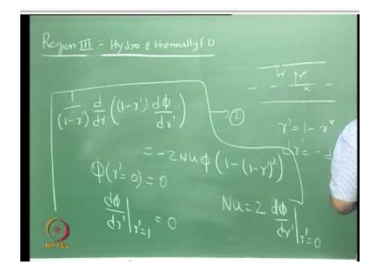
see now the coordinate system what you have been working with starts with the centre so what I would like to do is when you solve this with shooting technique you can start working from the coordinate system which starts from the w okay so why we can do that is that at the w you do not know the gradient okay also you do not the gradient is related directly to your nusselt number .
