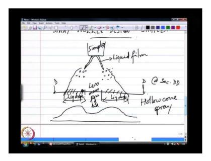
If I have let us say one of those simplex nozzle that I showed in the schematic and I create this film that is filling out this is the liquid film I am going to create this drops like assured in that same schematic here if I take a section down here call this I am going to have more drops. Let us say this is my spray now I am going to have more drops in this region and less drops here.
