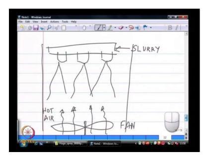
Like, I could have several nozzles that produce that spray this slurry and you have on the bottom side we have a fan that blows hot air. So, this slurry sprayed as it settles down to the bottom of a kiln of some kind, essentially loses it is solvent typically water and you start to get agglomerated granules, whatever particles where in a single drop now sort of agglomerate to form a cluster which gives you the feel of coffee granules.
