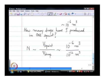
So, how many drops have I produced? That is simple that is the volume in each squirt divided the volume per drop that gives me the number. So, this is 10 power minus 6 meter cubed divided by 10 power minus 12 meter cubed. So, N is on the order of 10 power 6.
