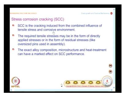
So, this explains what is the mechanism of crack growth by fatigue, now, we move on to Stress Corrosion Cracking abbreviated as SCC and we have already noted SCC is induced from the combined influence of tensile stress and corrosive environment; where do the tensile stress come about, see in many mechanical assemblies you have interference fits, these interference fits also can cause local tensile stress zones or if you have a oversized pin and that is what is summarized here.
