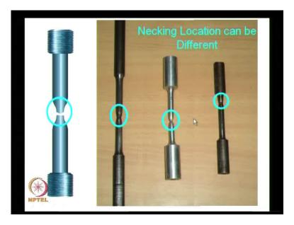
It is actually the internal flaw which dictate along the length of the specimen, where the necking would start and what happens is, you have a internal flaw which precipitates necking and this flaw grows in size that is what you see here, that is shown in red and after sometime you find suddenly on the ends you have a shear failure at 45 degrees.
