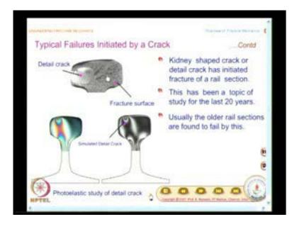
We had seen the variation of stress intensity factor on the boundary of the hole. It no longer remains constant. It is a three dimensional problem. The problem is very complex and you need to understand that. And, what is recorded is, the older rail sections are found to fail by this. And this has been the topic of study for the last 20 years, and the important aspect here is, crack has appeared below the surface. Here again, you see the crack surface and fracture surface.
