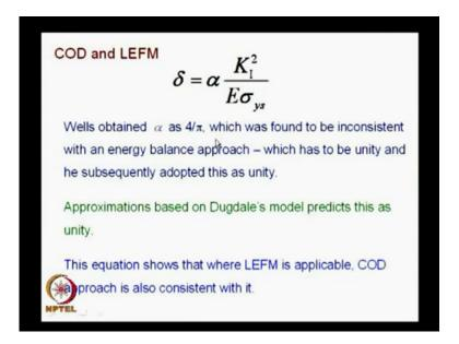
And you know I am not shown the derivations steps from Irwin's modified the value of the incremental extent of crack length it is possible to calculate an expression for the crack-tip opening displacement.
