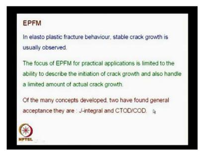
In elasto-plastic fracture behavior, stable crack growth is usually observed. I had mentioned, when there is crack growth, there is unloading. So, what people have put as their focus in EPFM was, for practical applications, it is limited to a ability to describe the initiation of crack growth, as long as you are able to achieve it, the purpose is satisfied and also handle a limited amount of actual crack growth.
