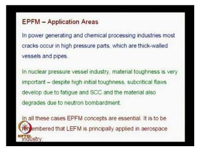
And we will see what are the application areas of EPFM, because people have gone for EPFM there must be a definitely need for it. In power generating and chemical processing industries most cracks occur in high pressure parts which are thick wall vessels and pipes.
