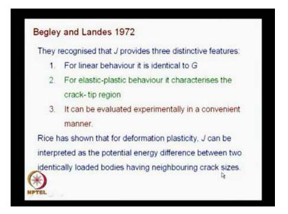
For linear behavior J is identical to G. So, that gives the comfort that we are going in for generalizations. For elastic plastic behavior it characteristics the crack-tip region like K determines the strength of the stress field linear elastic fracture mechanics in elastoplastic fracture mechanics J determines that the strength of the field is determine by J and another observation they have made it can be evaluated experimentally in a convenient manner.
