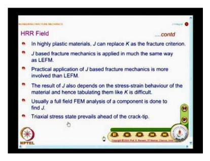
So, 1968 is a very important year from fractural mechanics point of view, we have important contributions that have been, made and let us look at, in highly plastic materials J can replace K as the fracture criterion.
