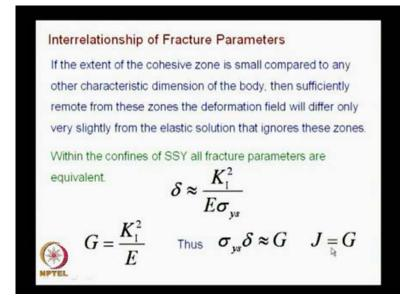
And in summary what you find is, if the extent of the cohesive zone is small compared the any other characteristic dimension of the body, then sufficiently removed from these zones the deformation field will differ only very slightly from the elastic solution that ignores these zones.
