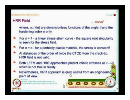
And this only summarizes what I had mentioned that sigma i j theta comma n are dimensionless functions of the angle theta and the hardening index n only. When n equal to 1 it represents the linear stress strain curve square root singularity is seen for the stress field.
