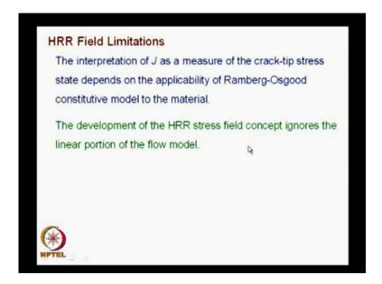
And if you look at the interpretation of J as a measure of the crack-tip stress state, depends on the applicability of Ramberg-Osgood constitutive model to the material and even in that what people do. In the development of HRR stress field concept the linear portion of the flow model is conveniently ignored.
