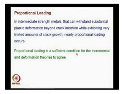
And this is again reemphasized. Proportional loading is a sufficient condition for the incremental and deformation theories of plasticity to agree.
