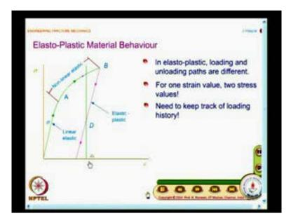
Now, I do an unload; it has reached a plastic condition and I unload; the unloading path is different. And what is its influence? Suppose, I take a strain value, two stress values are possible. You know, this is the very very key, important observation and this is where the complexity comes. When you want to go for plastic analysis, unless you keep track of the loading history, you will not be able to find out a relationship between stress and strain.
