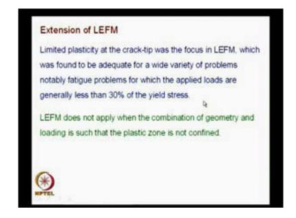
So, in such applications, linear elastic fracture mechanics would not be sufficient.
