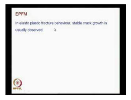
You have to take it with a pinch of salt. In elasto-plastic fracture behavior, stable crack growth is usually observed. And I have said, if there is a crack growth, unloading takes place. So, you have to find out, to what extent you can apply, the concepts of J.
