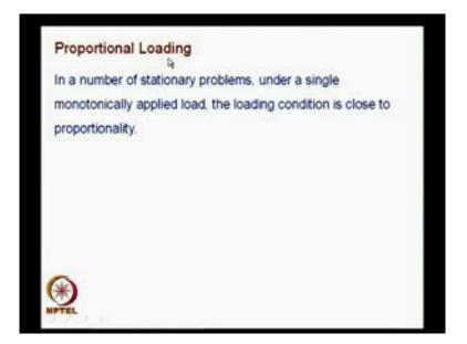
So, we have to necessarily make an approximation. In certain materials, you are able to see, that you will have more plastic deformation and very little crack growth; then, this is applicable. And here, you have a little more expansion on the terminology proportional loading. In a number of stationary problems, that means, crack is not growing, under a single monotonically applied load, the loading condition is close to proportionality.
