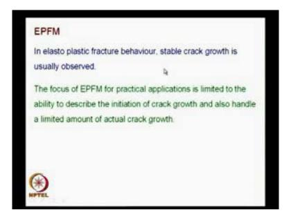
So, what we want to do is, the focus of EPFM for practical applications is limited to the ability to describe the initiation of crack growth and also handle a limited amount of actual crack growth.
