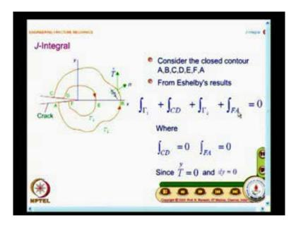
So, in essence, the integral C D and integral F A would go to 0; the reasons are stated here. Because it is a free surface, the traction is 0; and it is a very fine crack, so, dy equal to 0. Do not get misled by this V shape. This is, for illustration, it is put like this. So, when these two integral goes to 0, we get a very interesting result, integral over the contour 1 plus integral over the contour 2, equal to 0.
