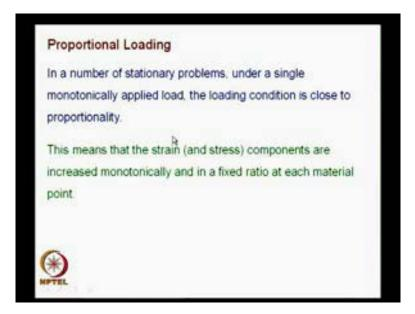
This means, that the strain and stress components are increased monotonically and in a fixed ratio at each material point. And this is how, you justify your approximation.
