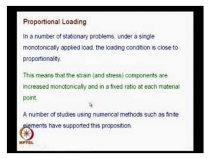
A number of studies, using numerical methods such as finite elements, have supported this proposition. See, the whole of elasto-plastic fracture mechanics, you have to look at proportional loading; that is how you justify the applicability of J, at least approximately. That you have to remember; it is not an exact representation. Approximate solution is good enough; as long as I am able to solve the engineering problems, even approximations are welcome.
