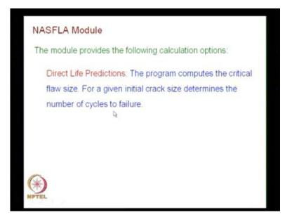
And if you look at, what are the constituents of NASFLA module, it can provide the following calculation options. You can do direct life predictions; the program computes the critical flaw size; for a given initial crack size, determines the number of cycles to failure. This is direct calculation. This is basic in any fracture mechanics calculation.
