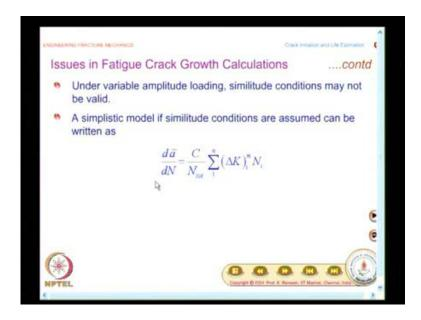
As I mentioned, variable amplitude loading is going to be very very challenging. And what you see here is, under variable amplitude loading, similitude conditions may not be valid. And you know, whenever we face difficulty, we will first come out with a simplistic model. A simplistic model, if similitude conditions are assumed, can be written as in this form. Instead of writing d a by d N, we write d a bar divided by d N;
