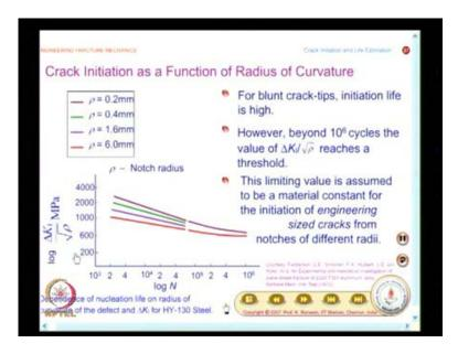
And, you also have this as a material property. Beyond 10 power 6 cycles, the value of delta K 1 divided by root of rho reaches a threshold; that is what you see here. The main purpose of this graph is, to show the delta K 1 divided by root of rho, reaches a threshold. And, people have found that this limiting value, is assumed to be a material constant, for the initiation of engineering sized cracks, from notches of different radii.
