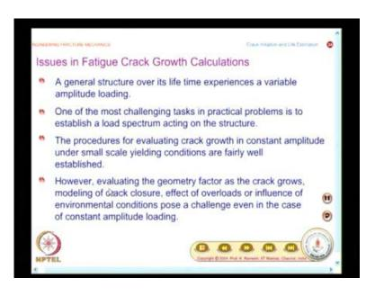
Evaluating the geometry factor as the crack grows. See, we have looked at stress intensity factor as K equal to beta times sigma root pi a and I said beta is the parameter which depends on the geometry of the specimen. And, when you have a crack and the crack starts growing, a by w ratio keeps changing. When a by w ratio keeps changing, you will have to find out the stress intensity factor, using several terms in the series. So,
