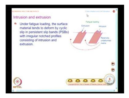
So, the roughness of the surface should change, which you would see by an experiment. And what you find is, the type of the intrusion, extrusion, whatever you see here, they are different, when you have fatigue loading and when you have monotonic loading. That is also recorded in the literature; that is what is shown here.
