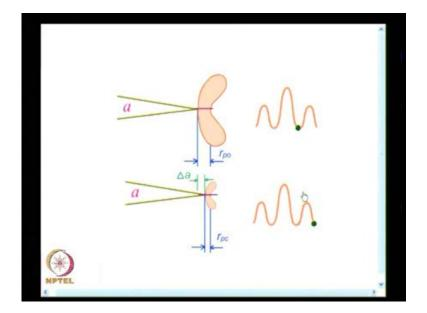
So, you have it here. So, I have the definition of these terminologies. I have a small crack length extension, because of one cycle of load; that is given as delta a. Mind you, these are all highly exaggerated pictures. These are very very small, when you look at the
