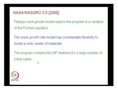
And if you look at, what is the fatigue crack growth model, that they have used, in the program, is a variation of the Forman equation.
