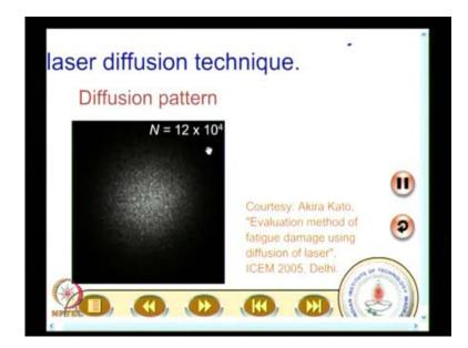
And when the cycle is increased, you see several dots. When the cycle is further increased, you see a large number of dots, indicating the extent of fatigue damage.
