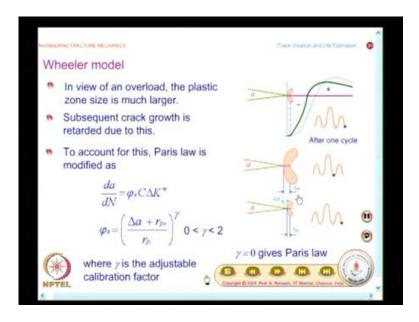
And, that is what is depicted here. You have along the crack axis, whatever is the length of the overload plastic zone is given by the symbol r p overload, that is o. When you have a normal cyclical load, the plastic zone is smaller. I think, I will try to magnify it; I hope it comes within the screen.
