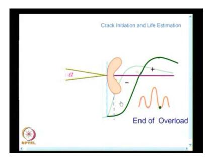
I have a smaller load followed by a larger load. So, for a smaller load, you have a small sized plastic zone; for a bigger load, you have a larger plastic zone. So, after an overload, you have only a smaller load, that is coming in the actual loading situation. So, the smaller load, will introduce on a small size plastic zone, but this plastic zone, will remain within the overload plastic zone.
