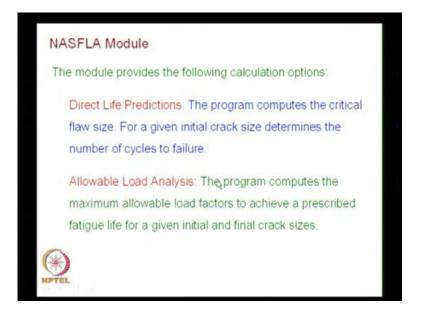
So, it can do direct life predictions, and it can also do allowable load analysis. And, what is the third aspect that we require. We need to know how to inspect; at what periodic intervals that you have to go and inspect. This is also possible in NASFLA.
