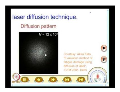
When the number of cycles increased to 12 into 10 power 4, the size of the diffusion pattern has definitely grown. So, this is an indication, that you have, slip bands are formed; the density of this fatigue damage increases after several cycles. So, this explains, that cracks can form at the surface and go beneath, and then, your Paris law
