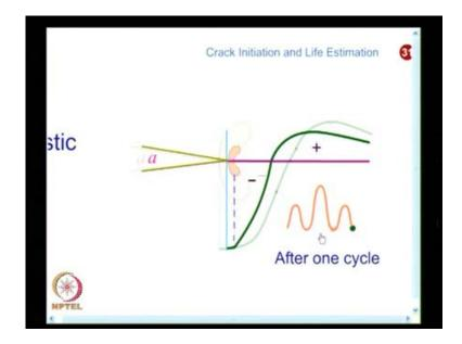
So, what we are looking at is, we are looking at, after the smaller load. So, I have this, crack has advanced, you have the smaller plastic zone, but this plastic zone, remains in the overload plastic zone. So, the rate of crack growth will not be as high as it was
