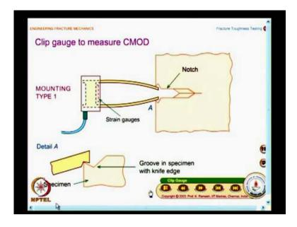
When you say you have to measure the load displacement, it is done by a clip gauge. People measure the crack mouth opening displacement. From your other transducer you get the load; from another clip gauge you get the crack mouth opening displacement. You know, this is where it is mounted to the specimen. Some detail is given; it could be mounted like this or it could have a sharp (( )) swivel type of edge and then you can have a detail like this.
