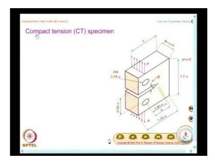
I said, this is the very popular specimen, mainly because, it is simple to fabricate and even the loading fixtures, to load it in the machine are easier to make.
