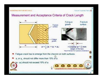
Then, as I mentioned, you also need to have, what should be the length that it comes out. The code says the fatigue crack has to emerge from the chevron on both surfaces. See, you see the crack length, only after the specimen is broken. You know, it is very difficult to measure the length of the crack as you do the loading; you have to have certain nondestructive type of measurement to see the crack has advanced beyond the chevron notch.
