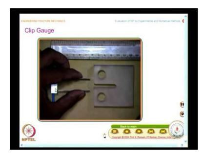
And in reality, what you do is, a clip gauge is taken and inserted into this; and this would measure the crack mouth opening displacement.
