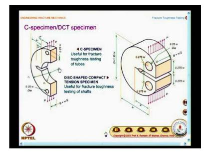
Then, we moved on to other forms of specimens that are used and I would like you to make a two dimensional sketch of this. This is a C-specimen.
