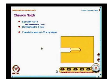
You know, in the last class what I had told you was, we have a diagram of chevron notch. There are certain restrictions the code gives; what should be the slot width, what should be the length of the slot and what should be the extension of fatigue crack. For all these, you have recommendations given. And usually, chevron notch specimen is shown like this. You have a line here; you have a line here; you have a line here and also 2 lines here.
