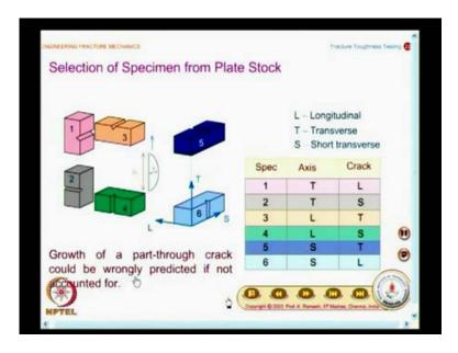
What is the consequence? The consequence is, growth of a part-through crack could be wrongly predicted, if not accounted for. This we had seen, even in leak before break criterion. I said a semi elliptical flaw would try to become an... from a, a semi elliptical flaw would try to become a circle, because K is very high and you want that crack to move further and create a leak in the pressure vessel; then, it should take some sufficient time for it to move sideways.
