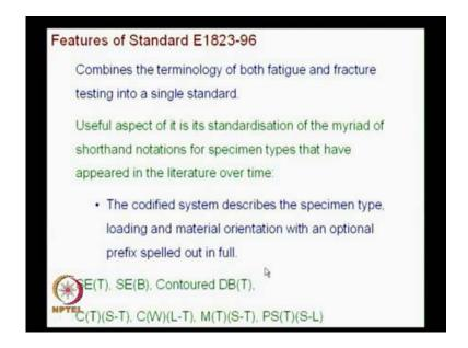
So, you will have something like S E within bracket T. So, this is nothing, but single edged specimen, with a tensile loading. When I have S E B, it is the single edged specimen with a bending loading. And you have a prefix, it is a contoured DB specimen. We have this double cantilever beam specimen; it is subjected to tension. Why it is contour? We have seen, if you want to have a constant K, you could design a specimen where the height of the specimen varies.
