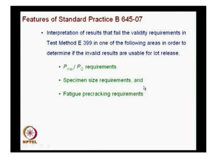
So, it is essentially like, how well a test can be salvaged? We will also see, what are the areas, if there is a fault in satisfying this P max divided by P Q requirements, what could be done? What is the specimen size requirements and fatigue pre-cracking requirements? So, if the conditions are not completely met, this provides a via media to accept some of them. It is not that, you summarily reject; is there any way you could salvage the test data?
