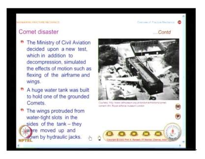
This flexing was not done because in flight, the wings alsocan flex because of the air currents, and it is a very quiet expensive experiment. As I mentioned, the wings protruded from water-tight slots in the sides of the tank. They were moved up and down by hydraulic jacks. So, it is more like a simulated fatigue test and an accelerated one, and they found a real surprise.Let us see what the surprise was.
