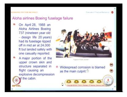
Now, we move on to another very famous accident. This is Aloha airlines Boeing fuselage failure, and this accident is slightly different. You know, in all the three other cases, we saw that the accidents took place very early in the surface, or within few years after the structure is built and put into surface. Here, it has happened after 19 years. The actual design life was 20 years.
