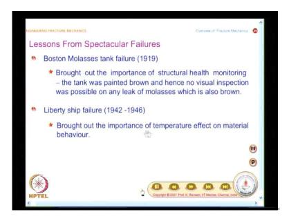
So, we had seen failures for the last70 years or so, in a span of 70 years, and what werethe main lessons from each one of these failure?Each one of these failure was selected to identify a particular improvement or cause that needs to be looked at in engineering practice.In the case of Boston molasses tank failure, it has brought out the importance of structural health monitory.You know, this is a very important aspect to see.
