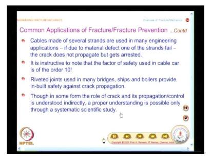
And if you look at, cables made of several strands are used in many engineering applications. Why you have cables made of several strands? It is for fracture prevention; if due to material defects one of the strands fails, that crack does not propagate, but gets
