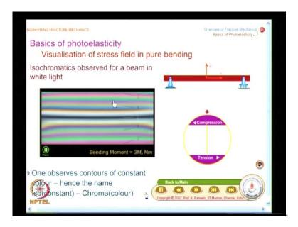
So, here, you have here, this is the beam.And what you find here is the value of the bending moment is progressively increased from 1M b to twice of that, and then thrice of that, and we will look at for this case.
