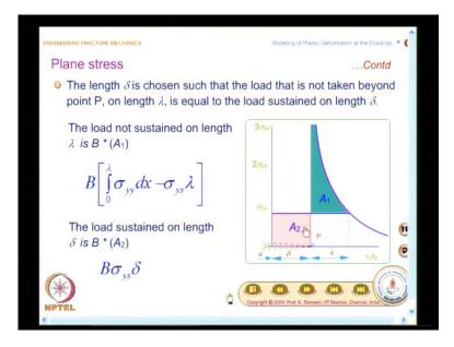
We have already seen the sketch, based on that sketch I can make a statement that length delta is chosen such that; the load that is not taken beyond point P on length lambda is equal to the load sustained on length one.
