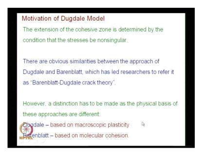
The extension of the cohesive zone is determine by the condition that, the stresses be nonsingular so, what I would appreciate is you go back and brush up whatever, the kind of stress intensity factor that we have developed for a crack subjected to symmetric loading. We will use that approach for us to find out the plastic zone length in Dugdale model, you need that expression. Go and brush up that, and come for the next class.
