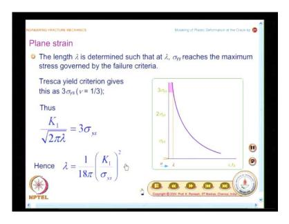
And you will also have to keep in mind that delta has a different symbolic representation when you go to EPFM, where it refers to CTOD rather than extension of crack length like this, we have looked at for plane stress now, let us see how do we estimate the plastic zone length in the case of plane strain?
