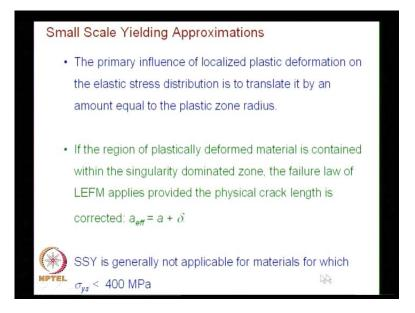
So, what you are really looking at it is, these zones are much smaller compare to the singularity dominated zone, that is the key point here. The primary influence of localized plastic deformation on the elastic stress distribution is to translate it by an amount, equal to the plastic zone radius.
