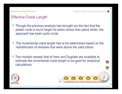
Now, what we will do is, we have already said that, we are going to model the plastic zone from further fracture calculation, by defining what is an effective crack length. The previous analysis has brought out the fact that, the plastic zone is much larger for plane stress than plane strain. However, the approach has been quite crude.
