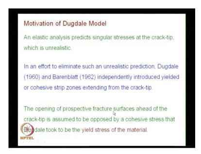
Now, what we will look at is, what is the motivation of Dugdale model? See, Irwin's model was very simple and straight forward, there has to be a need for another type of model and what way Dugdale have has approach. See, an elastic analysis predicts singular stresses at the crack –tip, which is definitely unrealistic, we did not have a choice so we were doing it not only that elastic analysis was very simple to do.
