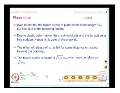
When there is no blunting in plane strain the sigma y, the maximum stress reaches the value of 3 sigma ys, which we find is not strictly correct, because of blunting, this was pointed out by Irwin. It is no longer 3 sigma ys was his argument, and what are the factors? Due to plastic deformation the crack-tip blunts and the tip acts as a free surface, I have already noted this down in earlier part of the lecture so, what you have is sigma xx is 0 at the crack-tip.
