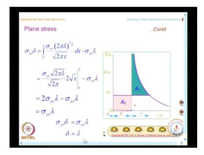
And you substitute this expression for K 1 in the above equation, and simplify. What we are really looking at is, we have to estimate what is delta. So, what you have here? I have sigma ys delta equal to integral 0 to lambda, sigma ys multiplied by 2 pi lambda whole power half, divided by root of 2 pi x dx, this is very simple to integrate, there is no difficulty at all.
