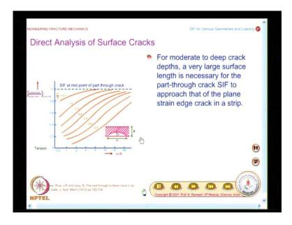
So, that is what is summarized here and the observation I had mentioned that the crack has to be long enough when the depth is more so that the stress intensity factor approaches that of the edge crack that is what is summarized here. For moderate to deep crack depths, a very large surface length is necessary for the part-through crack stress intensity factor approach that of the plane strain edge crack in a strip.
