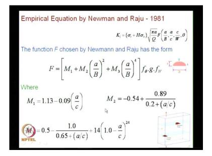
Then the function chosen by Newman and Raju has a form like this, f equal to M 1 plus M 2 multiplied a by B whole square plus M 3 a by B whole power 4 multiplied by a function of theta and a function g and function of w.
