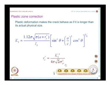
So, in a sense the surface crack is always more dangerous than a through-the-thickness edge crack, that you will have to keep in mind; though the stress intensity factor is a similar, but the fracture toughness we would use differently for a surface crack. And you know in the next chapter, we would discuss in detail how to calculate the plastic zone and as surface cracks are very important, people thought in what ways you could improve the results that we have obtained for surface cracks.
