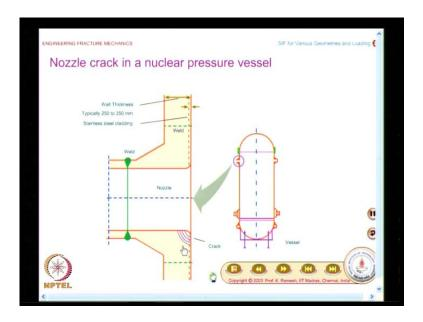
And in reality, corner cracks are very important. You know when you have a nuclear pressure vessel like this, you know the thickness of the shell is very high, it is about 250 to 300 millimeter thick, that means, it is a very thick steel plates; this is with a steel cladding that is what is shown here and you can have, when you have the nozzles from the corner, you could have corner cracks developed and these could be essentially quarter elliptical crack that kind of modeling is justified.
