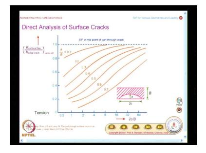
So, knowledge of stress intensity factor in a corner crack or a surface crack, they are all very important from practical design point of view. What we have now looked at is, if I have a shallow surface crack or a shallow corner crack, we know what is the way to get the stress intensity factor. And you know, people have also provided results in the literature on direct analysis of surface cracks, such results are also available and in those days people, where comfortable with graphs.
