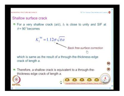
And people also have looked at, suppose I have a shallow crack, in a shallow crack I 2 is close to unity and SIF at ninety degree becomes simply 1.12 sigma root of pi a and we have already seen that what you have here is because of a free surface; you call this as a back free-surface correction.
