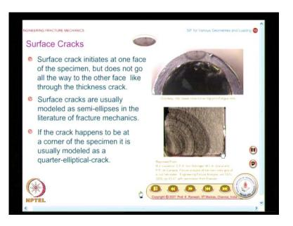
And what we will now see is from elliptical flaw, how do we graduate to surface flaws and this is where we had looked at in the previous class, how you will model the surface cracks. When you have a surface crack, the surface crack can be idealized as a semielliptical flaw to start with.
