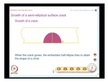
So, when it grows deeper, it is beneficial for us. Only based on such observations, people have also brought in a criterion call leak before break, which is achievable; this is how a material will respond. If you adjust your design parameter suitably, you can ensure that leak always occurs before break, because it is possible people have also evolved this as a criterion and we will see a nice animation which gives you this pictorially.
