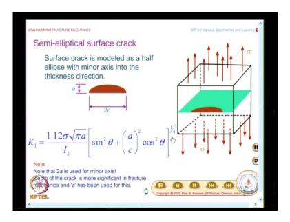
So, from the elliptical solution, if you modify with simpler arguments at least for small sized cracks, these results could be comfortably utilized that is how people have proceeded. When I have a semi-elliptical surface crack, you have to remind yourself the notational change.
