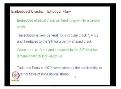
So the summary here is that an elliptical flaw would try to become a circular flaw. The solution that Irwin has obtained is termed as very general solution. For a circular crack the elliptical integral I 2 becomes pi divided by 2 and it reduces to the stress intensity factor for a penny shaped crack.
