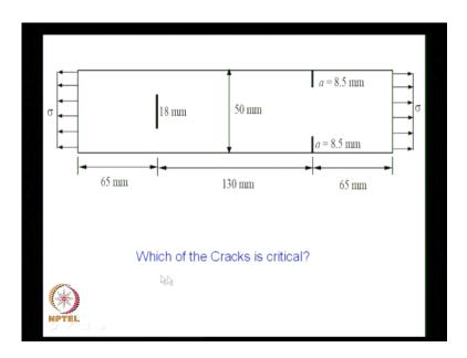
Now as you are having the equations just go back to that problem and then evaluate the value of SIF for a center crack as well as the double edge crack when the center crack is 18 millimeter and the double edge crack is eight point five millimeter. Double edge crack summation is shorter than the center crack.
