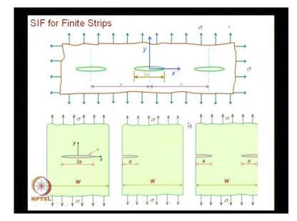
We have been looking at stress intensity factor for variety of geometries, and in the last class, we had looked at the problem of collinear cracks evenly spaced in an infinite strip. As I said, from an academic point of view, it would look like an extension of writing a stress function to a fictitious problem.
