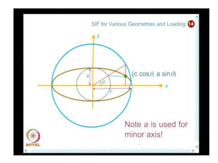
In the above diagram I have an ellipse and I have drawn a circle with the major axis and also drawn a circle with the minor axis.
