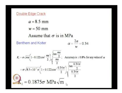
So in the double edge crack you have a equal to 8.5 millimeter, w equal to 50 millimeter and the expression of Benthem and Koiter. The value of alpha is point three four and after substituting it and simplifying the equation the value of K 1 is 0.1875 sigma MPa root meter which is definitely higher than the highest value we got for the center crack.
