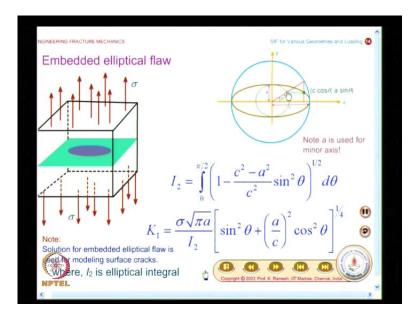
The stress intensity factor expression is obtained as shown here. The edges are given straight in the diagram but still consider this as an infinite body with in elliptical flaw. The value of K 1 is given as sigma root pi a divided by I 2 multiplied by sin square theta plus a divided by c whole square cos square theta whole power 1 by 4. Where I 2 is an elliptical integral which is in terms of theta . This primarily comes from how to locate a point on an ellipse.
