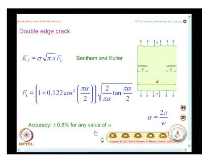
In the last class, we had looked at stress intensity factor for the center crack specimen as well as a single edge notch specimen. Now you have the solution for double edge crack with the definition of K 1 as sigma root pi a multiplied by the function F1. According to Benthem and Koiter, the function F1 is given as 1 plus 0.122 cos squared pi alpha divided by 2 whole multiplied by square root of 2 by pi alpha tan pi alpha divided by 2. Alpha is defined as 2 a divided by w.
