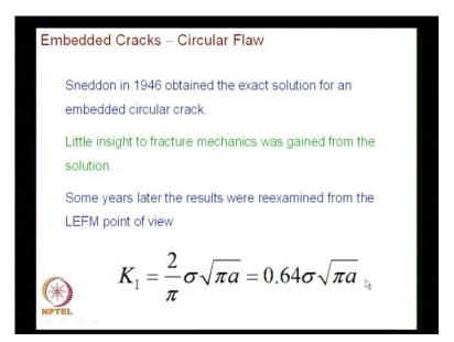
To summarize here, Sneddon in 1946 obtained the exact solution for an embedded circular crack. Little insight to fracture mechanics was gained from the solution. However, some years later the results were reexamined from the LEM point of view and you have got the result for K 1 equal to 2 divided by pi sigma root pi a written in another form as 0.64 sigma root pi a which is smaller than SIF for center crack specimen.
