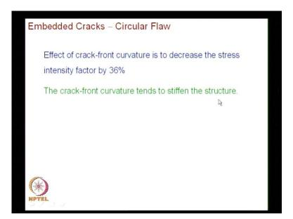
It is been analyzed that in the case of a circular flaw you have a curved crack front. The effect of crack front curvature is to decrease the stress intensity factor by 36 percent. In through the thickness crack, they could easily analyze the crack front and when they graduated to circular flaw fortunately the stress intensity factor was constant and was not changing. But after analysis they had brought in a conclusion that the stress intensity factor is reduced by 36 percent.
