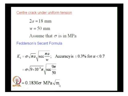
Now let us go to the formula by Fedderson's which is very famous secant formula and it is sigma root pi a multiplied by secant pi a divided by w. It is an empirical relationship based on heuristic arguments which gives you the value of K1 as 0.1830 sigma MPa root meter which is slightly higher than the tangent formula.
