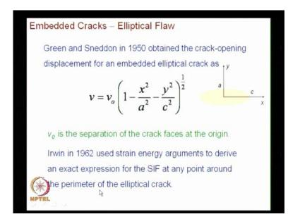
They initially obtained the crack-opening displacement for an embedded elliptical cracks as v equal to v naught multiplied by 1 minus x squared divided by a squared minus y squared divided by c squared whole power half, thickness crack the moment you come to embedded flaw and we would also graduate to surface flaw
