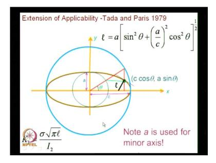
We have to go back to the diagram where we have identified the point on the ellipse for a given value of theta. According to Tada and Paris, draw a tangent at that point and drop a normal from there. Measure the length l of the line perpendicular to this tangent.
