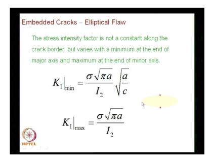
So first observation you get is the stress intensity factor on the elliptical front varies from point to point and you have a minimum as well as the maximum value. The maximum value of stress intensity factor which occurs on the minor axis decides which way the crack will grow. If you do the computation you find the stress intensity factor minimum along the major axis and it is given as sigma root pi a divided by I 2 multiplied by root of a divided by c.
