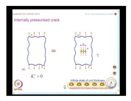
Now let us take a problem of internally pressurized crack. I have taken a simple strip subjected to uniform tension sigma and there is no crack in this. So when I do not have a crack I am justified in saying K 1a is equal to zero.
