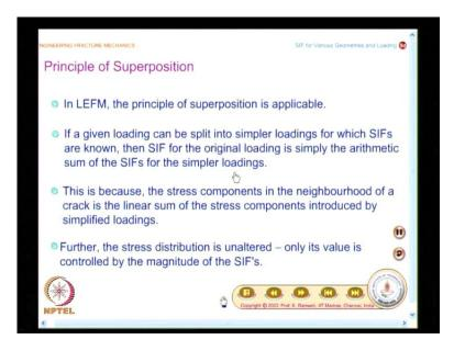
Another issue we have is about the critical crack which we will do by taking up another approach to SIF evaluation using the principle of superposition. Here principle of superposition is applicable because of linear elastic fracture mechanics. If a given loading can be split into simpler loadings for which SIF's are known, then SIF for the original loading is simply the arithmetic sum of stress intensity factors for simpler loadings.
