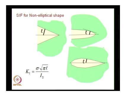
For different shapes measure the length 1 at the point you want to find out the stress intensity factor. Drop the normal and then find out the length 1 and if you have a smoothly varying type of situation put the tangent and drop the normal and find out the value of 1 then stress intensity factor is simply K 1 equal to sigma root pi l divided by I 2.
