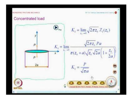
So, it is a very important problem, from that point of view. So, when I have it from concentrated load, this could also model for riveted hole, that kind of problems and you could also construct multiple solutions based on this. So, you have a problem like this.
