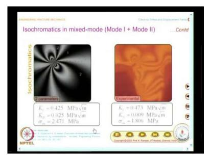
Here again, you notice, the 2 parameter solution is able to provide only the tilt; the size of the fringes are different; that is also captured. The tilt is different with respect to the crack axis. This is also captured by your 2 parameter solution. The 2 parameter solution is unable to capture the other features.
