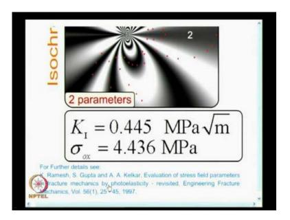
This paper has all the details. This is on Evaluation of stress field parameters in fracture mechanics by photoelasticity-revisited. Because this was the first paper, which utilized the equations of Atluri and Kobayashi and demonstrated it, its utility for a variety of problems. This appeared in Engineering Fracture Mechanics and there, you have the solution given as a function of number of parameters. All these fringe patterns are available.
