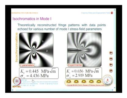
We start from a two parameter solution; we do not start from Westergaard singular solution. We said even for short cracks I cannot rely on Westergaard singular solution, I have to have minimum of 2 parameters. So, when I have minimum of 2 parameters, what do I observe? I only get forward tilted loops, and the fringes are not matching with the experimental data.
