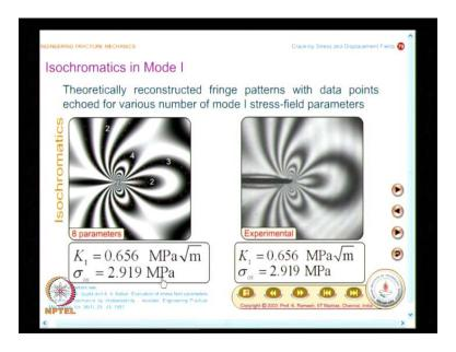
Simultaneously, also notice the variation, and the values of k 1 and sigma naught x; these are 2 pertinent parameters in the case of a mode 1 situation. So, I will repeat the animation. So, it is going for five parameters, at six parameters you know the contours match, you find sever and eight, there is hardly any change.
