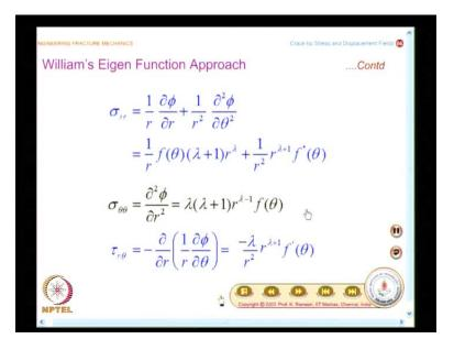
Now, let us brush-up our fundamentals in handling stress function in polar coordinates. If stress function phi is given, you can write sigma rr, and sigma rr is nothing but 1 by r dow phi by dow r plus 1 by r squared dow squared phi by dow theta squared, and we have already taken phi as r power lambda plus 1 function of theta, so, when I substitute this, the expression for sigma rr turns out to be 1 by r f of theta lambda plus 1 r power lambda plus 1 by r for theta.
