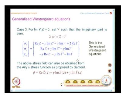
So, what you will have to look at is, by going to Irwin's formulation, we are able to enlarge a zone of data collection in the experiment. And finally, what Sanford pointed out was, you have to ensure only imaginary part of Y to 0; if you set 2 psi prime equal to Z minus Y, and you find the most general form of Westergaard equations, and this also models variation of fringe orders along the crack axis.
