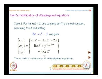
But, you will have to have a concept, that what way, this equation could be valid from an experimental point of view is, you are able to collect data, only a very small zone close to the crack-tip. On the other hand, in the Westergaard generalized formulation, if you set Y as a real constant, assuming Y equal to A and 2 psi prime equal to Z minus A, you get the Irwin's modification of Westergaard equation.
