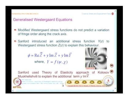
In the last class, we have looked at generalized Westergaard equations, and one of the key points in that was, we noted, that modified Westergaard stress functions do not predict a variation of fringe order along the crack axis. And this is the feature that you observe in an actual experiment. I have been showing these photo-elastic fringes for quite some time, I am sure you must be, now, very familiar in appreciating the fringe contours.
