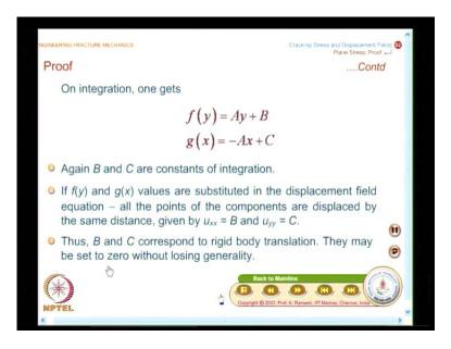
So, when I integrate this, I get f of y equal to A y plus B and g of x equal to minus A x plus C and these are constants; they are constants of integration. So, now, I know what is f of y and g of x; so when I substitute in the expression for u and v or u x and u y which ever way you look at it, I would like you to do that as an exercise in your rooms. I get u x as a constant B and u y as another constant C.
