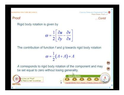
And now we look at what is rotation. The rotation is given a symbol omega that is nothing but one half of dou u by dou y minus dou v by dou x. So, the contribution of function f and g towards rigid body rotation is what you are getting it here, omega equal to one half of A plus A which reduces to a constant A. A corresponds to rigid body rotation of the component and may be set equal to 0 without losing generality.
