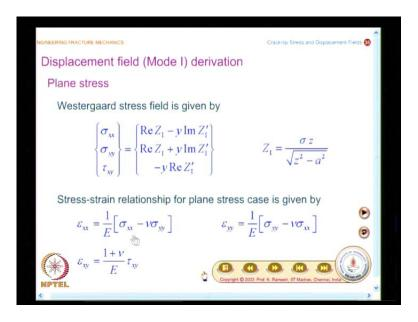
So, we go to the displacement field and here again what we will do is, we will develop it based on the stress function themselves and what is done here is since we are focusing on mode 1, the stress function given by Westergaard is represented as capital Z 1 and Z 1 prime and so on. In the earlier discussion, we had kept it as capital Z, because Westergaard used that basic solution to get the stress field for a variety of problems.
