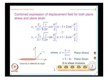
So, there is no singularity attached, when r goes to 0 what happens to these displacement components? The displacement components also go to 0. See this is another check for you to ensure that you earn the right direction. Your method of mathematics employed has been consistent, we got singular solution for the case of a stress field; we got a bounded solution in the case of displacement.
