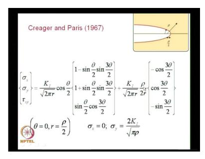
The crack-tip is not going to be sharp; in a real material, crack-tip would be blunt. So, people also looked at solution from a different perspective, this was done by Creager and Paris 1967, who tried to find out the stress field when you have a blunted crack-tip. How does the solution change? You had this Westergaard part of the solution plus you have K 1 by root of 2 pi r rho by 2 r multiplied by minus cos 3 theta by 2 cos 3 theta by 2 minus sin 3 theta by 2.
