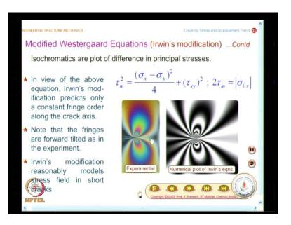
And we have also seen the kind of fringe patterns that you get by using this stress field equation; we will have a look at them again. We have calculated the maximum shear stress along the crack axes, turns out to be a constant value; this is the generic expression. When you plot these, you had fringe patterns like this, and when we compare it with the experimental fringe patterns, it matched quite well.
