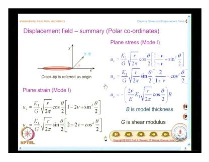
So, now, I have the expression of Z 1 as well as Z 1 bar in terms of r and theta. So, I can substitute it in the expression and get the displacement field in terms of r and theta as simple as that. And what is written here is I have the expressions for both plane stress as well as plane strain. In order to make your understanding very clear, the diagram reemphasizes that whatever the solution you see for the displacement field is referred to crack-tip as the origin.
