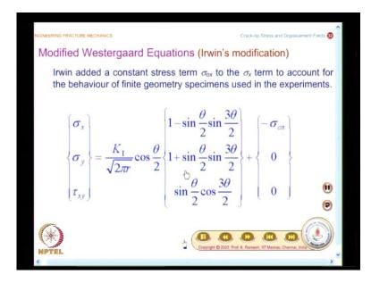
In the last class, we had developed the stress field equations and particularly we saw the stress field in the very near vicinity of the crack-tip; we have seen the solution by Westergaard; we also saw certain modifications on the Westergaard solution and one of the important modifications you have on Westergaard's equations is the modification by Irwin.
