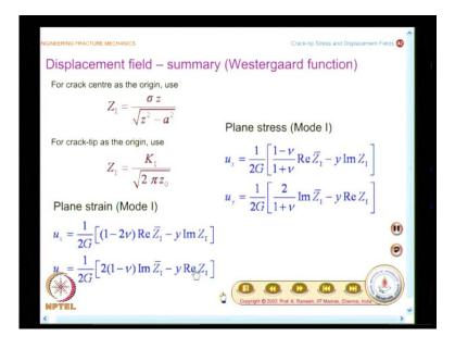
So, I can get referred with respect to the center using this stress function referred with respect to the tip with this stress function. So, essentially I will have to know, if I have to find out in terms of r and theta, I will have to know what is what is Z 1 and what is Z 1 bar. This is what I will have to do and this is just to verify your notes, it is all summarized here.
