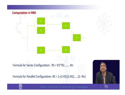
We will go to a computation of reliability block diagram. So, suppose this is the diagram. This is how things are connected say R1 and R2 are in parallel here. Similarly, the system somewhere it is in series somewhere it is in parallel. So, if we have to calculate the reliability then the reliability is if it is in series anything is in series. Say, here say for example, R4 and R5 has are in series.
