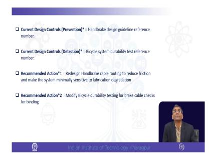
Current design control prevention, handbrake design guidelines reference number from some reference number it is given. Current design control, detection, bicycle system, durability test reference number. So, those are the reference number from which this details that information will be put in.
