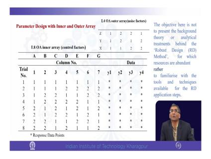
Now, here this is what you will see when you study anything in parameter design. I will soon after give the all the links where from. You can see this is this is combination of two arrays. One is L8 for the inner array or control arrays which Taguchi called inner array L8 or O8 and on top you find L4 or OA4 outer array which is the noise factors.
