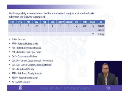
Here I will give you the glimpse I just said that that the format is available the slice of the format is presented here is that the first column is function, then is function that is function of the part what exactly it does that is the function of the part.
