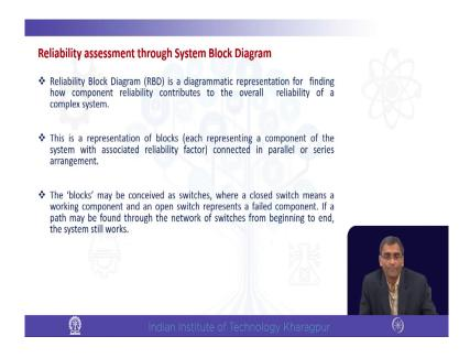
Reliability assessment through system block diagram, this is one interesting part that engineers or the designers mainly will have to assess the system reliability which actually is dependent on the component reliability involved in the system. So, we will see an example better than understanding or discussing theory.
