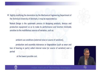
Now, slightly modifying another approach by the Mechanical Engineering Department of University of Denmark. I have put it because I have liked it because it is very to the point robust design is systematic process in designing products, devices and production equipment so as to make its performance and function minimally sensitive to the multifarious sources of variations.
