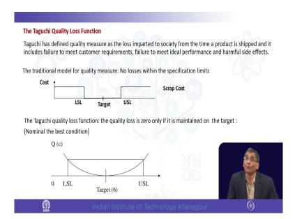
So, in Taguchi's loss function here you see the traditional model is there is a upper specification limit or lower specification limit. The target is in between because if it crosses the upper limit we reject if it crosses the lower limit you reject, that is very well you have learnt in your studies earlier.
