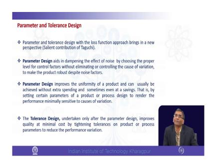
Now, parameter and tolerance design I have already discussed that. Parameter design aids in dampening the effect of noise by choosing the proper level for control factors without eliminating the control controlling of the cause of variation and we have said. And, it improves the uniformity of the product.
