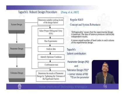
The definitions are everywhere I am not spending much time on the definitions you can see that and this is also the steps I have already explained that first is system level, then there is a parametric parameter design then tolerance design. And, here the orthogonality means that the experimental design is balanced.
