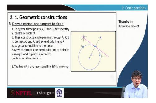
The first question that we will ask is if there is a circle on how to draw normal and tangent to that circle from a given point. In certain instances, we might be having only three points. So, using three points, first of all, we have to construct a circle then we will be in a position to identify the centre and then radius, once radius is done we will pick the point, normal direction vector we will write and also the tangent direction we will be in a position to do. Let us do that step by step.
