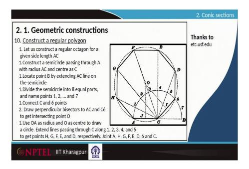
Let us construct a regular polygon; for example, we will like to make an octagonal polygon constructed from AC given side. So, the AC side is given for us and the same AC length we would like to have it on other sides. To construct that, let us look at the procedure. So, what is given is AC length is given as side length. First of all, we have to construct a semicircle passing through A with radius AC and centre as C.
