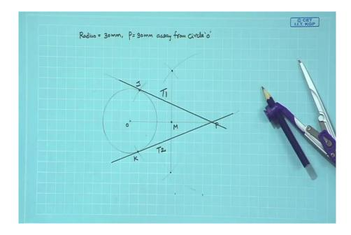
Let us pick radius of the circle as 30 mm, the point P for through which we will construct tangent is something about 90 mm away from circle centre O. So, first let us take the scale to pick a point, let us call that point as O P point is 90 mm away from centre O.
