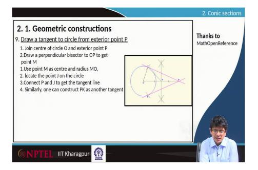
Let us look at the second problem. How to draw a tangent to a circle from an exterior point P? So, here what is given is there is a circle having a centre O, passing through points J and K with a specified radius, and there is an external point P. From point P, one has to draw a tangent passing through J or K. To do that, let us look at the procedure. First of all, what we have to do is join the centre of circle O and exterior point P, so that circle is given,
