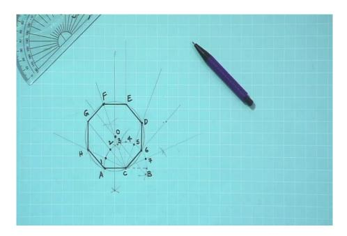
So, let us pick an example. With AC as side length, we are going to construct an octagon. So, it is supposed to have 8 sides AC side length is a 20 mm side we would like to construct.
