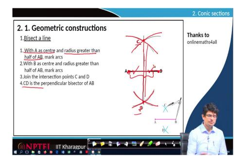
Let us look at the steps involved in constructing this bisecting line. The first step is to draw a line AB and then with A as centre; so here we will use our compass; keep it as a centre and radius greater than half of AB; the distance from A to B is that. So, perhaps I pick this much radius, which is more than half of AB. Use compass from here, construct an arc; with the same radius from point B, also using a compass, I will construct one more arc.
