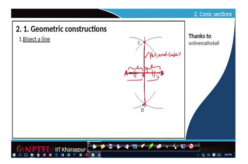
The first objective is how to bisect a line; here there is an AB line with points A and B. For this line, we would like to bisect into equal parts; that means if I am calling this point as O; AO distance and OB distance are equal to each other and that we construct it based on another perpendicular line.
