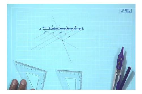
First of all, we have to draw a line, mark A and B points, draw an inclined line. Now on that line, pick radius an arbitrary one; mark these points, so use this point; let us mark this one, pick this one as centre; mark the second point. Similarly, use that one as centre; mark the other one.
