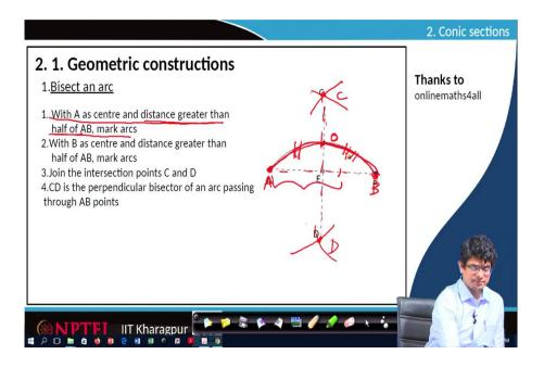
So, AO and OB are equal. Let us look at the next object 2; how to bisect an arc? Here we have an arc A to B; the first point is A, and the last point is B, and we would like to bisect this arc; that means, this point let us call O; AO arc length along the arc and OB arc length supposed to be equal.
