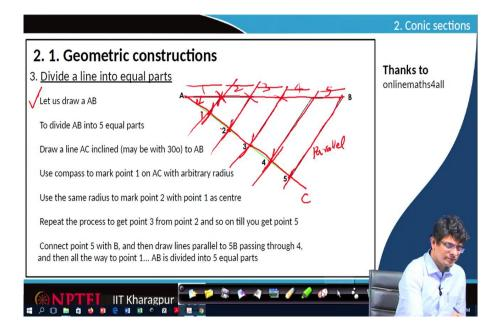
The third point objective for our today's session is; divide a line into equal parts. So, let us consider there is a line AB, and we would like to divide that into equal segments; perhaps 1, 2, 3, 4, 5 equal segments we would like to construct. The procedure to do this: after drawing line AB, draw an inclined line AC; this is the line, perhaps an acute angle like 30 degrees, 40 degrees, and so on to AB.
