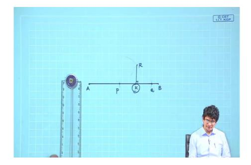
Let us first draw a line AB; maybe this is the line; let us join it. Call this point A, call this point B; now mark a point K somewhere here, and we would like to draw a perpendicular line through geometric construction.
