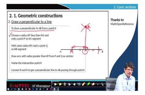
Let us look at the procedure; first of all, draw a perpendicular to AB from point K. This is the object to what we have to do. The first step is to choose a radius KP less than KA. From K point, pick another arbitrary point P such that AP is smaller than PK, so something like this is the greater distance.
