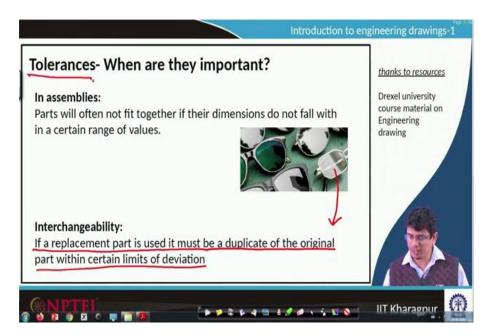
For example, you broke your one of the glass; you would like to replace it this one you would like to replace it. If a replacement part is used, it must be a duplicate of the original part within certain limits of deviation.
