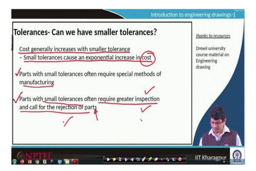
It is a common practice cost generally increases with smaller tolerances small tolerances cause an exponential increase in cost to make it. Parts with smaller tolerances often require special methods of manufacturing, its not only about cost if you are going for very small tolerance values to prepare that itself we require special equipment.
