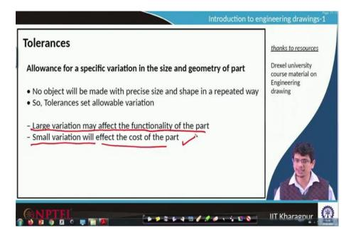
Now, all these dimensions for drawing are perfectly fine like saying 12 mm, but if we ask a machinist to prepare 12 mm kind of object, perhaps it can be the length it can be hole its not possible to precisely make 12 mm. There are always be plus or minus deviations possible because we are dealing with machines, there are many factors which influences this machine.
