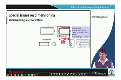
So, from here it is 22 mm up to this portion and thread perhaps the object size is up to that hole might be created up to this level, but threading is done up to this level only. So, in that case, the thread length 18 mm also has to be shown this is the 18 mm. This is the way threads and special screw features are shown.
