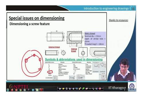
Usually we go with symbols for any kind of dimensioning by just looking at that symbol, we will be in a position to understand whether the drawing consist of diameter or spherical diameter radius and so on. If we are using phi it represents diameter, if it is something like S phi its indicates that spherical diameter.
