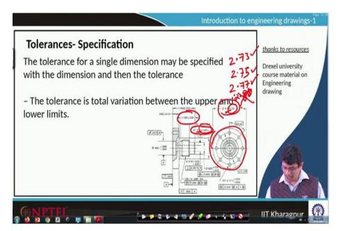
Let us look at an example here we have a drawing sheet on which there are many components mentioned, for example, its a for a turning operation the chalk screws and other things here is represented, for example, let us pick this one. We can see that something like phi representing diameter 1.375 units with plus or minus 0.005 units.
