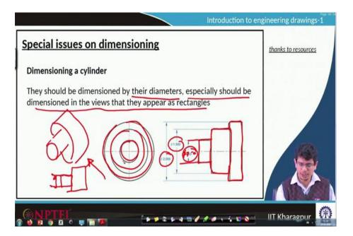
On special issues on dimensioning in the last class, we looked at different ways of dimensioning it. For example, if it is a cylinder having multiple steps. So, that on the other side of the view we look at like a step one, try to look at diameters if it is diameter we use symbol phi, and smallest one inside and the largest one outside that is the way we try to look at.
