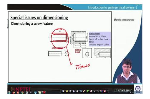
Similarly, if we have thread screws, etc., we do not put threads directly on that for dimensional purpose and other things. We show particular dimensions that indicate that these are threads.
