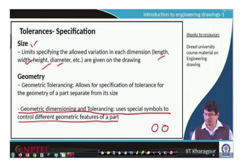
We specify these tolerances in different ways; for example, it can be based on the size it can be based on geometry also. For size, let us look at it. It limits specifying the allowed variation in dimension; that means, it can be length width, height or diameter etcetera are given the drawing. These kind of things if we are talking about those are about size tolerances regarding geometry also we talk about this tolerances.
