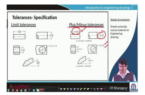
And these tolerances are broadly divided into two parts one is limit tolerances, where we show the dimension 2.5 2.45 both the things. Similarly, limit tolerances for which limits are mentioned it can vary from 1.4 to 1.5, this diameter can vary from 1.5 to 1.75 and so on so things.
