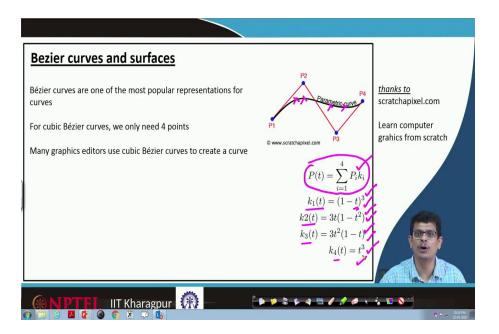
If I am representing it in terms of parametric variation the P any point P, on that curve the parametric curve supposed to be expanded in terms of P i k i where k 1 k 2 k 3 k 4s have these cubic interpolations. So, t is our parametric variable, like our u, a cubic polynomial, a cubic, a cubic, a cubic in different kind of formats we are going to carefully adjust. So, that we will be in a position to construct polygons, through which this particular polynomial curve really passes.
