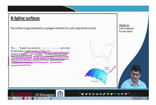
The other way of representation, these data points trying to construct surfaces called B-splines, which is also called as basis splines technique. Because it is a drawing course we are not going too many details into the mathematical formulation of these curves, but just to have an overall idea about what kind of curves are good for what kind of applications, that is the thing what we are going to learn about it.
