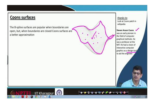
The other kind of surfaces is Coons surfaces. Especially, the B-splines the basis splines are popular when boundaries are open, you have discrete data points, but these discrete data points are not forming any boundary. Somewhere inside of that object you have it then you use B-splines, but if these data points on one particular kind of boundary. We employ these Coons surfaces and this Coons surfaces are better approximations.
