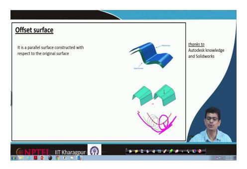
Now, we are going to draw a tangent there so that means, we have that point. So, now, join those points construct an offset surface. This is the easiest way one can really construct any offset, if we want to really improve the quality of that curve, we use specialized curves.
