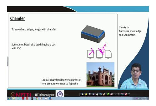
There is another terminology also we use when we are constructing these 3D objects using software, which we call chamfer.
