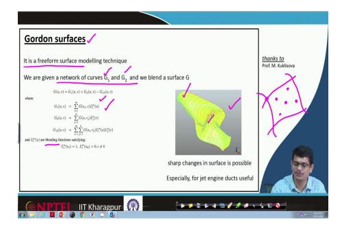
The other kind of representation is by Gordon surfaces. So, these kinds of Gordon surface is called freeform surface modelling, that means, you have data points you can really drag-drop, so that surface is naturally adjusted on that CAD software.
