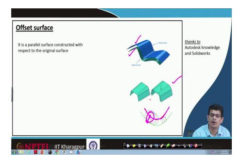
Here, we have some asbestos kind of sheet, the roof a parallel thing we would like to construct, that is what we call offset surfaces here also. One way of the easiest way of looking at that is, this is the curve or surface what we have first construct a point in that normal to that direction, draw a circle with one particular radius, wherever that surface is a tangential point pick it. Something like, we have a point here with an offset distance as radius draw a circle.
