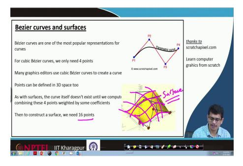
If you are looking that in 3 dimensions. For example, this is the first data these are the 4 data points, we have. Then first, we will construct a Bezier curve in that. Similarly, we will be having other data points like one perhaps, two at bottom three and four then again we will be in a position to pass another Bezier curve. Similarly, another Bezier curve, another Bezier curve similarly on the other directions we have 4 data points. So, pass a surface a Bezier curve in that way.
