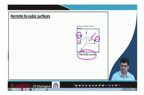
The first one, in terms of Hermite bicubic surfaces, what we do is we construct a curve between points. Those points, if we are joining if we are getting a specialized curve, for example, the point p0, p 1 we know these are any x y coordinates of that system.
