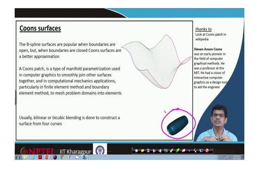
A Coons patch, is a type of manifold parameterization used in computer graphics to smoothly join other surfaces together, and in computational mechanics applications, particularly in finite element methods and boundary element methods, you would like to really mesh the problems of domains into elements and so on. These Coons surfaces are quite popular.
