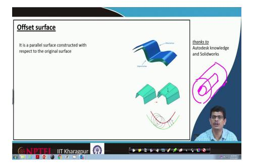
Similarly, in a CAD software, we use other variety of surfaces, named offset surfaces. You have one surface with respect to that one surface with an offset, similar kind of surface we would like to construct it. For example, I have a cylinder, let, for example, I have a cylinder. I would like to have one more concentric cylinder around that if I am going to construct such kind of thing that is what we call this offset surfaces.
