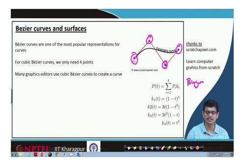
There are other ways of constructing surfaces also, those are called Bezier curves and Bezier surfaces. In that, we have particular data points like P 1, P 2, P 3, P 4. We do not straight away join these data points, what we do is we construct based on certain, polygons fit in between these data points. And when we are fitting these polygons, whatever the curve which passes through that crossing these polygons that is what we call Bezier curves.
