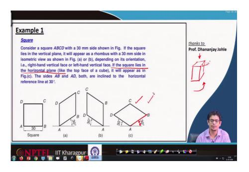
If the square lies in the horizontal plane, like the top face of a cube; we are looking from the top and that plane is on the horizontal plane, it will appear as figure c. We can view it in different directions; but when we are representing it in the isometric plane, we have to rotate in such a way that or we have to shift our position in such a way that, one of these principal edges makes 30 degrees angle with the plane, that is the way we have to represent any isometric projections.
