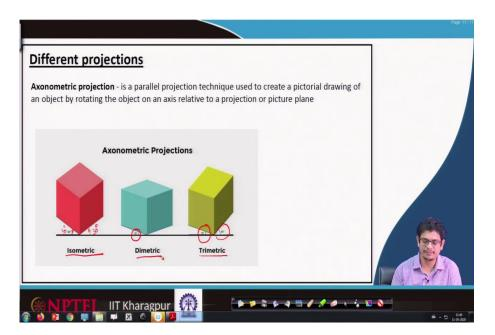
So, under these different projections, we have seen axonometric projection; it is a parallel projection technique used to create a pictorial drawing of an object by rotating the object on-axis, relative to the projection or picture plane.
