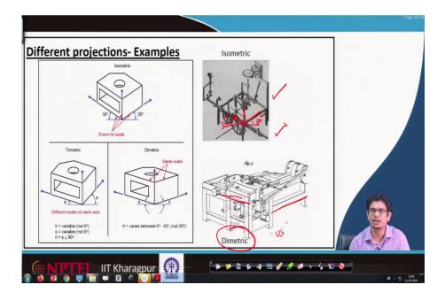
Just an example, we have an object here for isometric view; if we are fixing some of them as axis, for example, this is one axis, this is another axis, this is another axis.
