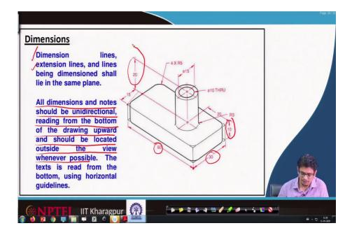
Regarding dimensions when we are showing, dimension lines and extension lines; these shall be on the same plane.
