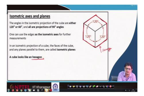
If we are taking a cube in the isometric projection, we sense it like a hexagon; so, let us look at these edges; these are the standard conventions when one supplies drawing sheets for the protection thing.
