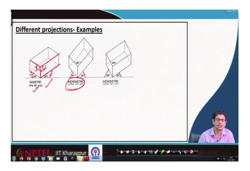
Here we are showing different projections of this rectangle by a rectangular (Refer Time: 25:51). So, for example, in the isometric view the box; we will represent it in such a way that, it will be rotated in such a way that one of these principal edges makes a 30-degree angle.
