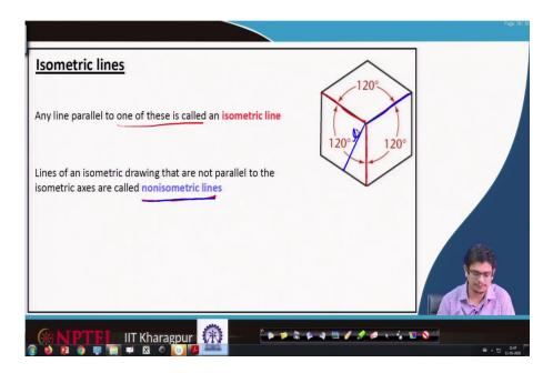
Any line parallel to one of these edges is called isometric lines; this is one isometric line, any line parallel to that also isometric lines. If we are drawing a line, not parallel to these isometric axis; we call non-isometric lines.
