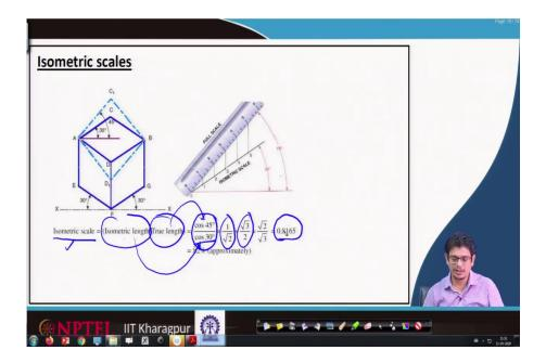
So, the isometric scale defines such kind of terminology, where we are going to compare isometric lengths with the true lengths. So, when we are looking at isometric lengths, it always makes on this x-axis 30 degrees; though axis make 120 degrees, when we are measuring with respect to the horizontal, it makes 30 degrees.
