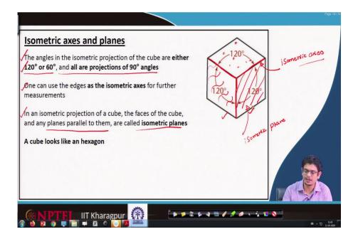
Now, we will look more about isometric axis and isometric planes. The angles in the isometric projection of the cube are either 120 degrees or 60 degrees based on how we are defining and all are projections of 90 degrees angles.
