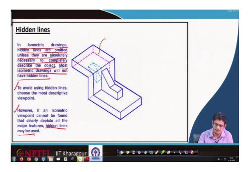
Regarding hidden lines when we are representing on isometric projections; in isometric drawings, hidden lines are omitted unless they are necessary to completely describe the object. Most isometric drawings will not have hidden lines. If you are opening any isometric projections; we usually do not show those hidden lines, unless it is very important to show.
