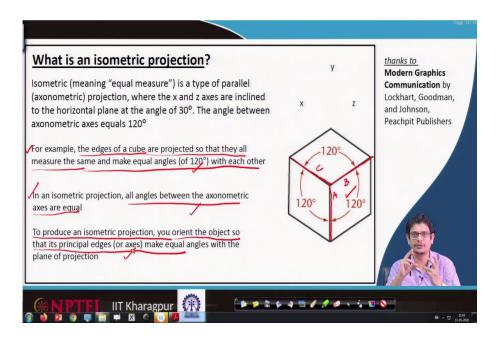
For example, the edges of a cube are projected so that they all measure the same and make equal angles 120 degrees with each other. That is the first thing for the isometric view.
