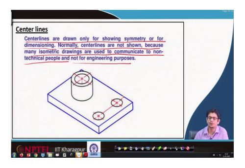
Now coming back to centre lines. Centre lines are drawn only for showing symmetry or for dimensioning point of view. Normally, centre lines are not shown; because many isometric drawings are used to communicate to non-technical people and not for engineering purposes.
