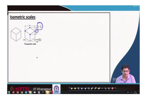
And note that in the isometric, this angle always is 120 degrees. Similarly in the perspective views if we are going to compare; for example, this point to this point let us call length h, and this point to this point let us call w and if h by w is equal to 1 over root 3.
