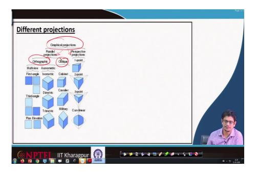
So, the different projections, typically the entire engineering drawing graphical projections can be mentioned as parallel projections and perspective projections. And in parallel projections, we have orthographic projections and oblique projections.
