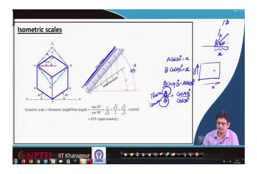
For example, if we are taking a cube here; we use a scale named isometric scale, this is defined as isometric length to true length. So, the cuboid might be having unit dimensions in reality. When we are representing it on a paper in the perspective of isometric projection; the object size may not be one unit length, it changes, usually it changes to 0.82 times of true length.
