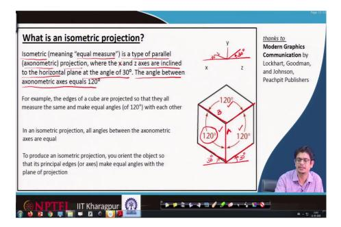
Now, we will learn more about this isometric projection in detail. Isometric means equal measure; here equal measure angles we will have it.
