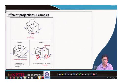
In the dimetric view, we have theta angle on both sides and this theta angle varies in between 0 to 45 degrees and this is not 30 degrees. So, we always have this object, for example, like if we have this object; we have to rotate this object in such a way that, different views we are going to see.
