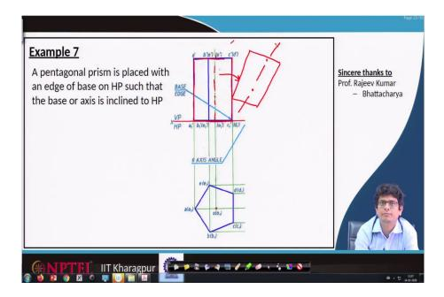
Now, what we want to do is rotate this entire object in this direction. That means, basically the axis what we are having, dash-dot line this has to be rotated in that direction. So, all this line has to be rotated in that direction. This entire line has to be rotated in that direction and this one also in that direction. In that way, if we can make it our axis goes in that way.
