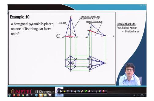
Once we know that this length which is in the middle the same thing, we can connect it so that we can make that triangle. Once we have that transfer this point projections vertically down.
