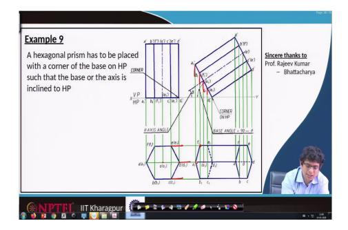
Now, project these points from top view on the from the front view and also from this direction. From here transfer the points, so that it intersects. So, one has to be careful.
