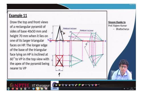
Let us take another example. Draw the top and front views of a rectangular pyramid of sides of base 40 by 50 mm, is a rectangular pyramid. There is a reason you have different sides different lengths 40 and 50 mm and it has a height of 70 mm.
