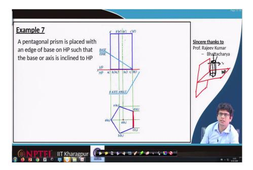
So, one of the edge, we make sure that it will be perpendicular to the vertical plane. So, it is more like if we have this prism first what we will do is we construct in such a way that this entire prism, so in the top view we will see something like such kind of thing, so where the axis is perpendicular to HP.
