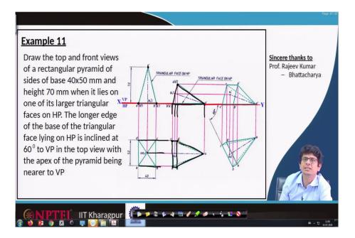
So, what we will do? o to b' first of all we locate it on that horizontal plane. Then, transfer this a point precisely to that location. Then, project all these points down. Similarly, project these points, then we will have the pyramid. In this way, it looks like in the top view. The remaining things are dashed lines.
