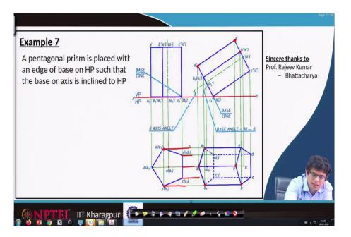
Once that is done, we transfer all these points onto the horizontal plane, down. So, these point these points transferred in such a way that this line maps to that, this one maps to that and whatever the b b 1 point and so on.
