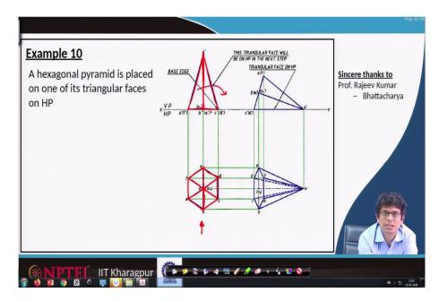
Let us take one more example. It is a hexagonal pyramid. Pyramid means we have this apex or vertex and it is placed on one of its triangular faces on the horizontal plane.
