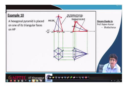
If I am rotating it in that direction this o' c' edge has to be resting on the ground. So, o' c' we draw it. Measure o to c', locate o' c', draw that. Now, transfer this a d' in this way. From here measure the thing whatever that length makes an arc, because this entire thing; from here also measure this one; make another arc. So, once we have that point connect this by the triangle.
