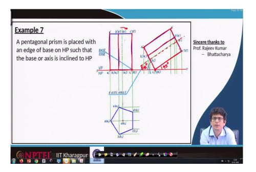
So, when we do that, first of all, we draw an axis making certain inclination angle maybe if it is making 45 degrees, at 45 degrees first we draw an axis. It is rotated about this point. So, this point always is resting on that; using our compass whatever this distance that distance we make an arch, perpendicular to this axis and join that line.
