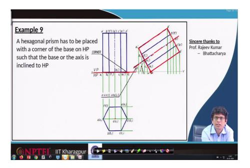
And axis is inclined to that horizontal plane which we can sense it only in the front view. So, the axis dash-dot line. Transfer all these lines, so that we will see, this one. If we are carefully noting corner of that base is always be resting on the horizontal plane, that is the reason we made it to rest it on this horizontal plane and this corner still rests on that horizontal plane. So, this point always is on that ground.
