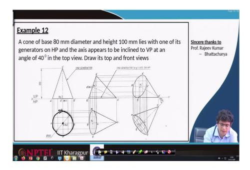
Now, let us look at the loss example. Here a cone of base 80 mm diameter and height 100 mm is lying with one of its generators on the horizontal plane. So, a cone generator has to be on the horizontal plane and its axis appears to be inclined to the vertical plane.
