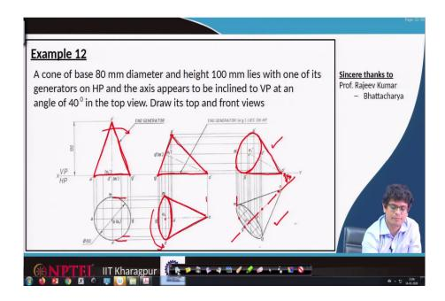
Have a front view which looks like a triangle, then rotate it in such a way that one of the generators may be og' resting on the ground. So, use once we draw og' resting on the ground, we can always locate a point by compass.
