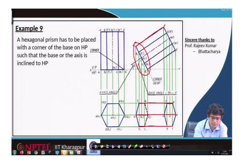
And this one is visible. So, we have a continuous line. These edges are also visible that is a reason these are continuous lines.
