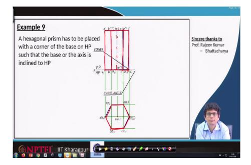
Now, let us look at another example. A hexagonal prism has to be placed with a corner on the base of the horizontal plane, such that base or axis is inclined to the horizontal plane. Think about it what are the points resting on the horizontal plane, is the axis incline with the horizontal plane or vertical plane. In what sense? And the corner of this hexagonal prism of that base is on HP. So, let us look at that example.
