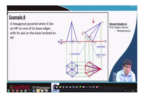
Now, identify the lines which are visible when we are looking from this direction will be seeing a' o o' lines that means, a to o will be visible. Similarly, f' o' that face also visible. So, it will be that. Definitely, a to f' whatever this line we can see that is also visible.
