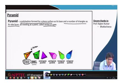
After prisms, there is another object what we call pyramids. A pyramid is a polyhedron formed by the plane surface as it is base and a number of triangles as it is side faces, all these should meet at a point called vertex or apex. For example, let us take a triangular pyramid. We have these triangles all these are meeting at 1 point, this one is apex or vertex.
