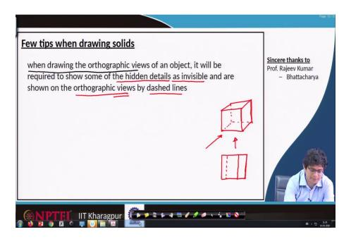
So, when we are drawing these solids, there are a few tips which we have to follow. Especially, when drawing the orthographic views of an object, it will be required to show some of the hidden details as invisible. That gives us a feeling that it is not a two-dimensional object, it is a three-dimensional object. And, these are shown on the orthographic views by dashed lines.
