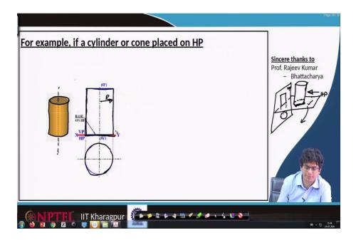
Now, let us ask a question if a cylinder or cone is placed on a horizontal plane, how it looks like, what are the projections for the solid? So, let us consider this cylinder. It is a solid object; the axis is that. Now, this cylinder is placed on a horizontal plane. So, again construct our 3 D picture. This is the vertical plane, this is the horizontal plane, and what we have is cylinder resting on the horizontal plane.
