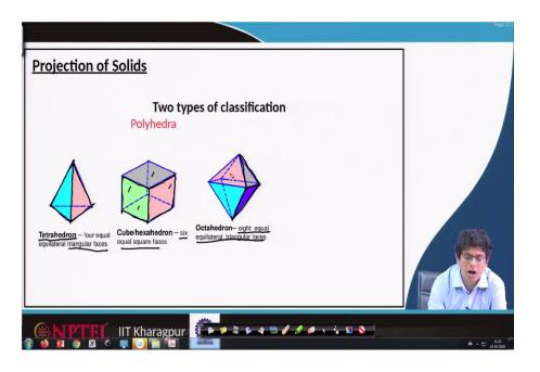
In polyhedra, we have different varieties like a tetrahedron, cubes, and octahedron. So, if we are looking at this object tetrahedron. We have four equal equilateral triangular faces. So, this is the first face, the second one and third and fourth faces. So, in that way we have this tetrahedron fourth faces.
