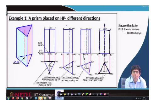
Let us look at this example if a prism is placed on a horizontal plane; however, at different directions. So, this prism is always be placed on a horizontal plane, but one of these edges making different inclination angles if so, how it looks like? For example, one of the edges on the base, because this is the one, which is placed on this vertical plane, no horizontal plane.
