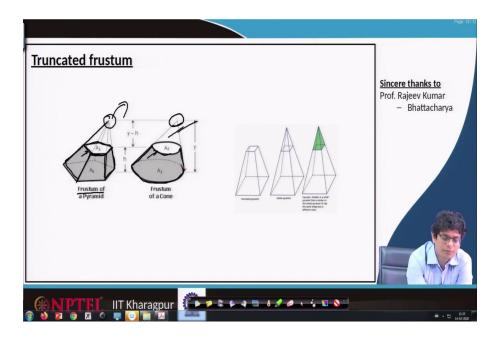
If we have a pyramid take a slice, this is the pyramid it might be right angular kind of thing vertically making 90 degrees. Half perhaps slightly slanted one, if we are taking a slice at this level passing a plane taking a slice of that it makes a frustum. So, there is a leftover part, what we call frustum?
