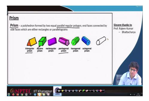
Similarly, there is a different kind of objects which are called prisms. A polyhedron formed by two equal parallel regular polygons, end faces connected by side faces which are either rectangles or parallelograms such kind of objects what we call as prisms.
