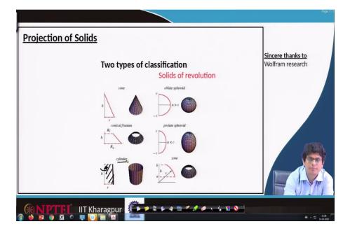
Similarly, a line revolves around this axis give us cylindrical surface; a plane rectangular plane revolving around that axis gives us a cylinder.
