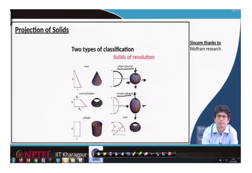
Similarly, if we have curves, for example, this curve, it can be semicircle it can be slightly elongated semicircle also if we revolve it ellipsoidal kind of objects we will get. And, usually, we call these are spheroids from spherical geometry we construct them.
