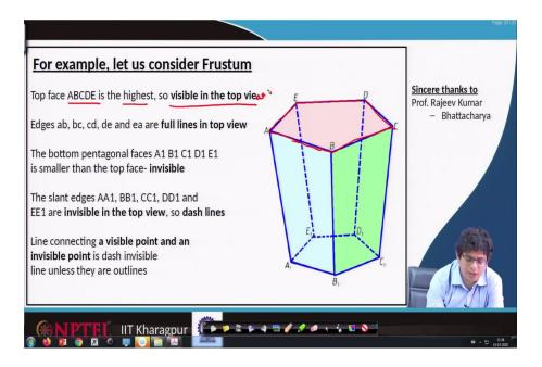
For example, let us consider a frustum; that means, some part we have removed it. Frustum by definition it might be having a cone or pyramid kind of shape or perhaps pentagonal thing. And, one part we have removed and the part what we have removed is apex side of the part. That means, in this case, the size of this pentagon is very smaller than the size of this pentagon.
