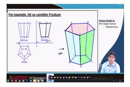
Let us take the top view. So, the top view we are looking at from that direction. So, X Y plane, a horizontal plane like, what we have guessed ED, AE, AB, BC, CD are visible. This is always visible, inside one not visible, not visible line. Similarly, when we are looking A to A 1 there is a line this one. So, let us use some other color.
