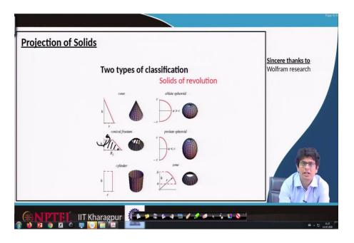
For example here, this is the line which is at a distance R 1, and R 2, if this line we revolve it, it makes a peripheral surface in that way. Which is what we call conical frustum? If it is a plane this entire plane revolves around this axis, then we will get a conical frustum of a solid object; that means, the material will be filled inside also.
