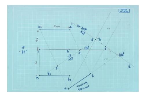
First of all, let us draw an X Y plane. This is the X-axis, Y-axis. Draw the top and front views of one of the ends. Say a 45 mm above HP. So, this is a vertical plane and this is a horizontal plane, 45 mm above HP let us locate it. From this point 45 mm, this is the point and 60 mm in front of the vertical plane.
