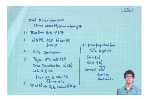
Let us summarize this entire thing. The first step for this problem, draw the top and front views 45 mm above HP and 60 mm in front of VP. These lines let us assume that both are parallel to HP and VP. Now, construct a line inclined at 30 degrees to HP that gives us auxiliary inclined plane which is making 30 degrees angle with respect to our horizontal plane and this is perpendicular to vertical plane also.
