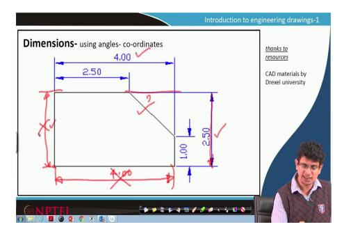
In the next example, we will see when we are going to represents those angles. These basic dimensions 2.5, 4.0 and this one, 0.25 are good enough to represent this incline portion. Because we are already showing this 2.5 in this way, we don't require any dimension here.
