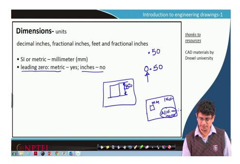
For drawings, SI or metric units precisely speaking millimetres we represent. Usually, technical drawings always consist of it takes mentioning all dimensions are in mm, such kind of text we usually incorporate
