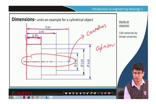
In this case, what we are trying to look at is from this view we are trying to look at. So, that this part is this part and this part we are looking as this one and this part is that is rotated by 90 degrees object, that one what we are trying to look at. So, it is a cylindrical one. That is the reason; we have these dash, long dash, followed by a short dash, followed by a long dash, short dash and so on. This kind of lines we call centre lines.
