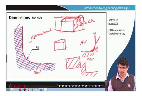
If there are arcs involved in that, one has to be careful in showing these dimensions. For example, you have a room floor where edges are slightly corner. Because there is material on this side, this is the room air, and this is the room material, these are the edges. So, whenever material is there, we show it by this kind of hash lines. This indicates that material is there, and there is no material on this side.
