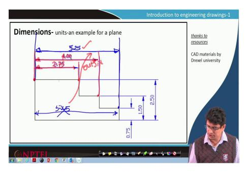
In this drawing, there are dimensions something represented from here to here whatever that length is available representing by a line, arrowheads and number 5.25 one of the basic dimensions. From here to here whatever length is there that's represented by 4 units. From here to here that line is 2.75.
