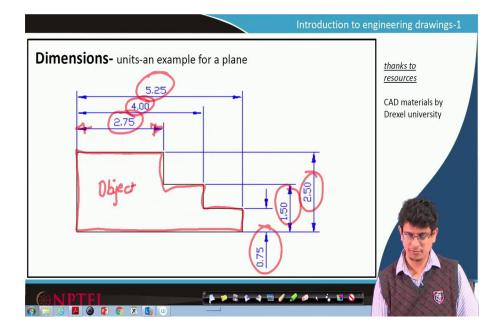
This is the object what we are looking at is a stepped one, and the dimensions are these continuous lines with arrowheads.
