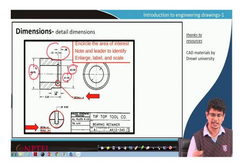
And the other basic dimensions, what we can see is here this. Because it is a cylindrical object, so we have a diameter as dimension and so on.
