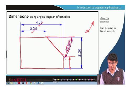
For the same example, if I would like to use inclined angles. So, for the same object the 2.5, 4, but we do not want to represent this height or length, instead of that what we are trying to do is this is having an incline, incline with respect to this horizontal line. So, we are showing it as an inclined angle. So, we are using this angular thing mentioning our 45.00 degrees. So, this is 45 degrees.
