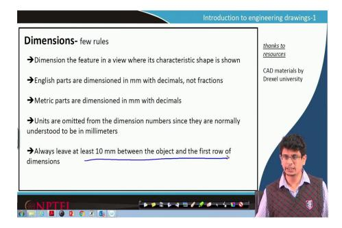
Few rules, dimension the feature in a view where its characteristic shape is shown. So, the main features have to be conveyed through these dimensions. English parts are dimensioned in mm with decimals, not
