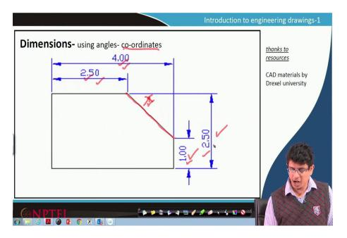
Now, because it is an inclined cut section, we may require an angle. So, there are two ways to show these angles. If we are strictly following Cartesian coordinates, it's better to use just numbers without showing any angular coordinate.
