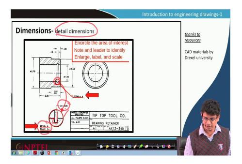
For example, let us look at this one this small red one, that one extensively we are showing it at sides the side of this drawing sheet. So, we want to mention those intricate dimensions also that is the reason we are showing it as a separate one with clear cut dimensioning it is having R of 0.05 units, and that is what we call detail dimensions, any intricate things which we would like to specifically show, then a separate thing like rounding it off into circle and show it.
