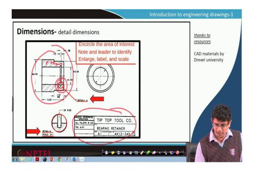
These dimensions supposed to be in detail, one has to show. For example, here we are taking a drawing an example drawing sheet where an object is mentioned, the title block perhaps the material is present there that is the reason this hashing is done and the intricate details we would like to show.
