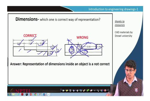
Let us recall our discussed rules. The rule it is breaking, one should not show dimensions inside of that object that is a wrong thing and the minimum 1-millimetre gap from the ah 10-millimetre gap one has to use from the object, in this case, these are followed because the object is in this level. So, these dimensions are away from that object, but here the dimensions are within the object. So, this is a wrong representation.
