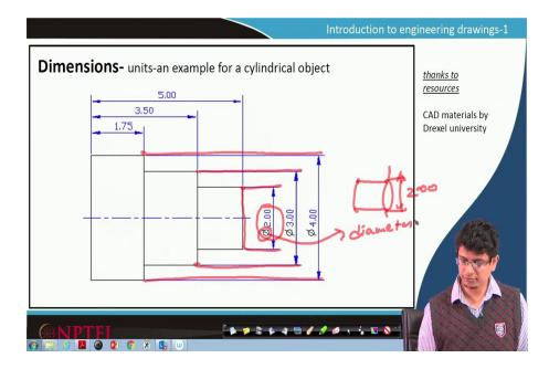
Instead of showing the gap between step to step, what is that gap we are not showing, but what we are showing is what is that diameter, what is the diameter for that step, what is the diameter for that step we
