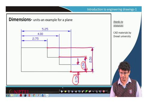
The next one is from here to here this height, the projection height vertical thing this is 1.5. From here to here, that is 2.5.
