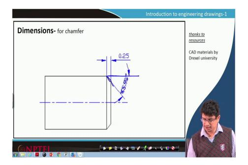
So, because it is a chamfer, we are showing 45 degrees, for example, and that is from that chamfer to this reference base, this is the reference base. So, that angle what we are showing as 45 degrees. Because it is a cylindrical object that is the reason we have a dash-dot line.
