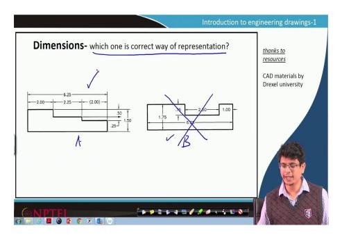
Let us close this a session with the last example. Here, I am showing you two pictures, two different pictures A and B, which one is the correct way of representation. Let us look at picture A and picture B. Picture B is the wrong way of representation when compared to picture A why?
