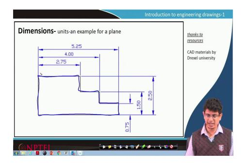
Let us understand dimensions and units using an example for a plane figure. Here we have a staircase drawing; for example, this is the staircase given as a drawing.
