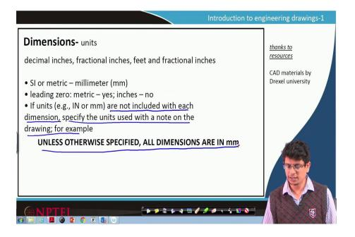
So, as I said units are not included with each dimension, specify the units used with a note on the drawing as unless otherwise specified, all dimensions are in mm. This is one kind of template to represent units.
