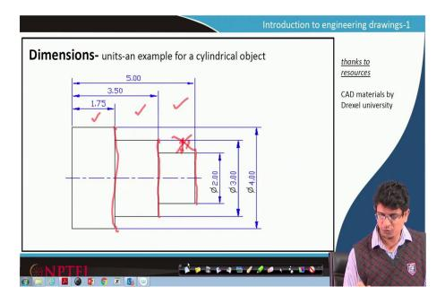
Now, because it is a cylindrical object, there are certain dimensions associated in this direction also. It is a cylindrical object; usually, the diameters matter a lot.
