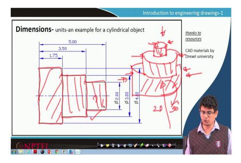
Instead of a plane object like a 2D object, if it is a cylindrical object, let us look at it. Here, we can see that the object on the sheet looks like that with lines. Later lectures, we will understand how to construct such kind of things, what exactly this entire object represents, but in this class, we will learn about dimensions.
