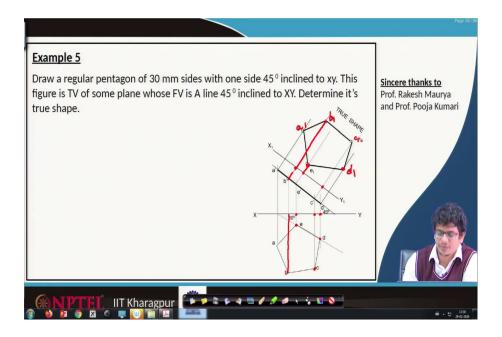
From the XY axis, this is the one from all the way to b this distance we will transfer it from this point to that point let us use some other colour, the red one. So, this length from XY axis to be that line we will project it from X 1 axis here to b 1. So, already we have projected from b 1, on that we use that length to identify b 1 similarly a 1.
