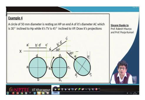
Once that is done, this plane has to be rotated by 45 degrees and thus, inclined to the VP. So, once we have this kind of ellipse, what we are going to do? That ellipse entirely we are going to rotate it in that direction. So, that in the vertical plane, ah top view we can see that rotation.
