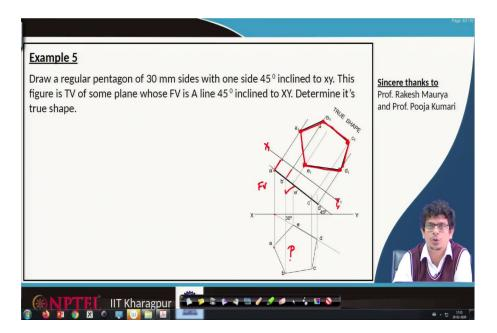
Once we have these points a, b 1, c 1, d 1 and e 1, we connect it to get the true shape or original shape of that object. So, our auxiliary plane method, when we know the front views and the top views in this case, ah front view is giving us a line with true line and the top view is after ah having this view, we are getting a pentagon of regular shape.
