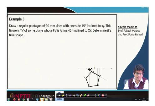
Now, let us look at a new example. Here, there is a regular pentagon of 30 mm sides with one side is 45 degrees inclined to XY axis. This figure is a top view of some plane whose front view is a line 45 degrees inclined to XY. If that is the case, determine its true shape.
