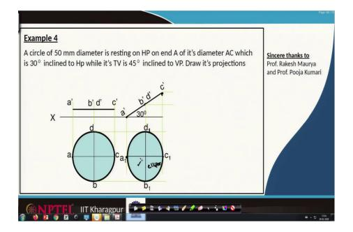
Once that is known, now we have to make 45 degrees angle that how we are going to make it is projected these lines, first of all, a all the way to a down, c all the way to c, b and d. Now, a if it is mapped to a 1, d mapped to d 1, c to c 1, b to b 1. So, when we ah lift this by 30 degrees, the complete circle looks like an ellipse, it looks like an ellipse here.
