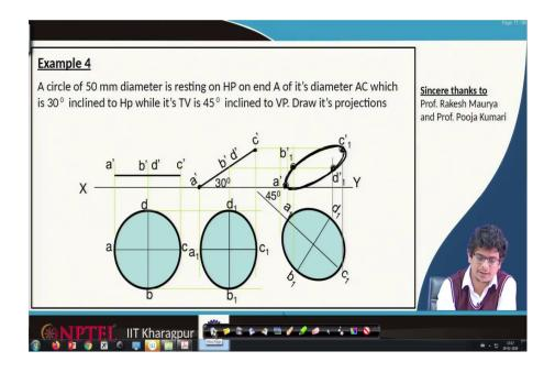
Correspondingly, the b 1 points, d 1 points are also mapped. Then, we will we can have these projections. Once we have this a 1, b 1, c 1, d 1 the way how we rotate is this ac line from here through that we are going to make it 45 degrees so, the projections always give us this a', b 1', c' and d' through that we have to draw a freehand sketch which makes an ellipse.
