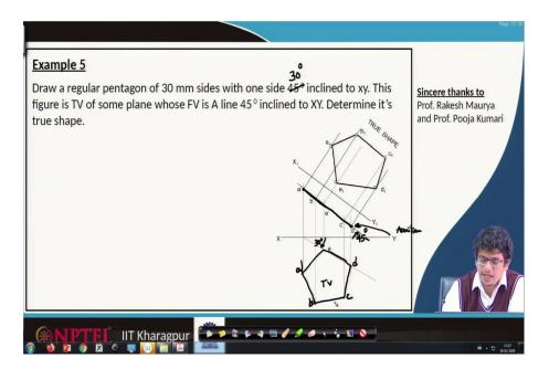
Let us take an example, look at these steps. For example, on this slide, draw a regular pentagon of 30 mm sides with one side is 45 degrees inclined to XY axis. If that is the case, first of all, we draw a pentagon is regular pentagon 30 mm side. So, this is one of the views given with 30 mm side, we draw a pentagon. We draw it in such a way that one of the sides makes 30 degrees angle.
