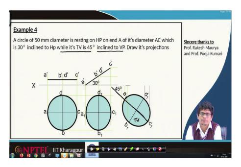
While its top view. So, this is the top view that has to make 45 degrees inclined to the vertical plane. So, this entire ac line supposed to make 45 degrees. So, we rotate it in such a way that we will get this 45 degrees line.
