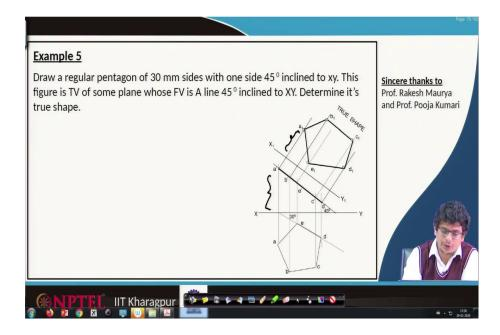
So, a' to X-axis whatever the distance, the same distance from X 1 axis so, this distance and this distance are the same. That is the way we transfer these lengths.
