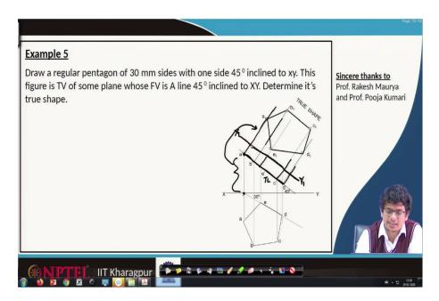
Mark this points a, b, e, c and d on this line. So, those are the thing. Now, we have to draw X 1, Y 1 parallel to this true line. So, parallel to the true line, we are drawing this X 1, Y 1 axis.
