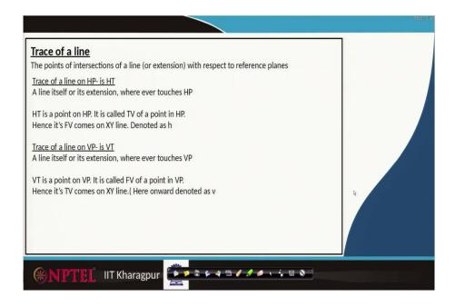
So, the point of intersections of a line or their extension with respect to the reference planes is called traces of a line. And there are a different kind of traces of a line with the horizontal plane and also vertical plane.
