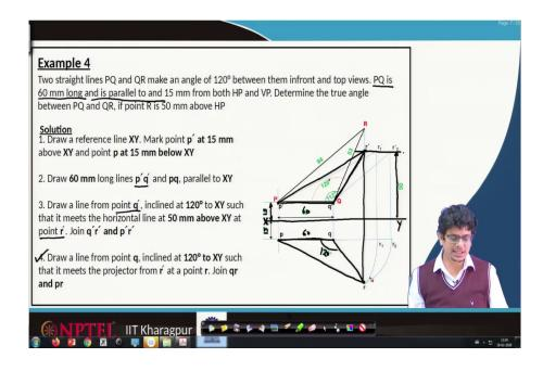
So, let us solve that problem step by step. First, draw a reference line XY on the plane, then mark a point p' 15 mm above HP, so this is 15 mm above that HP. In the front view, we are projecting that 15 mm, so that p' point will be at 15 mm.
