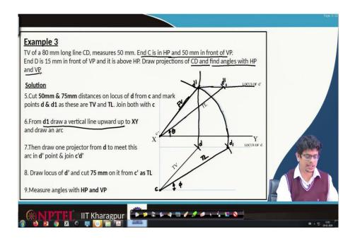
Once that is done, we have to make 50 mm and 75 mm distances on locus d from c. So, this is the c point locate 50 mm cut and also 75 mm cut, because end C is in HP and 50 mm in front of the vertical plane.
