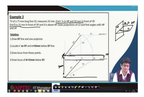
Let us begin. The third example is there is a top view in that 75 mm long line CD which measures 50 mm, and its end C is in the horizontal plane and 50 mm in front of the vertical plane. End D is 55 mm in front of a VP and it is above HP plane. If that is the case draw projections of CD and find angles with the horizontal plane and vertical plane. Let us look at the solution.
