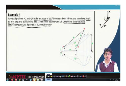
Now, let us solve one more problem for our projection of lines. So, let us look at the slide, here example 4; there are two straight lines PQ and QR. So, it is not just one line, but two lines PQ and QR, they make an angle of 120 degrees between them in front and top, in the front views and top views.
