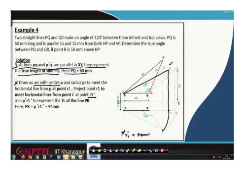
Once this construction is done, look at this step 5. As lines p q and p' q' are parallel to XY, they represent the true length side of PQ; here PQ is 60 mm. Now, we have to draw an arc with centre p from here, and radius pr that is this p to r, so that we can locate a point r 1; so, in this direction, we locate r 1.
