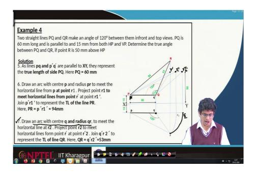
So, after drawing this p' r', p' r' and also p' r 1' connecting these points. Now, we will move on to seventh point; where we have to draw an arc with centre q and radius q r that is from q r radius to meet horizontal line at r2. So, with this radius, if we are going in this way we will locate r2, then project this r 2 all the way to locate r2'.
