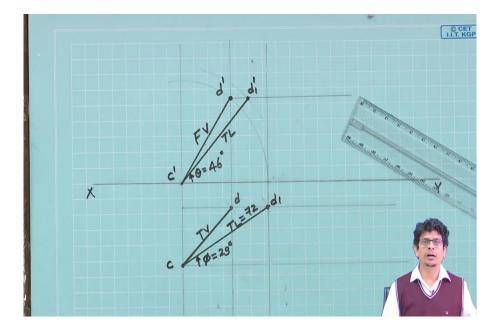
So, on the drawing sheet first, we have to draw a horizontal line XY; name this x-axis, y-axis. And draw a vertical line to locate this projector this is the projector, and our c' is already on the X-axis, XY axis so c'.
