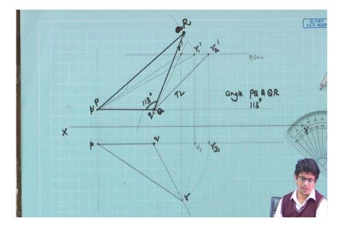
First, what we have to do, draw an XY line; X-axis Y-axis. Then mark points, so draw a projector line which is 15 mm above XY, locate that point p' lower case letter. Similarly, 15 mm below this one also, so let us call this point p. Draw horizontal lines, locus lines both from p and p', these are the projected lines.
