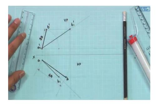
This is the XY line. The first step is to identify true line 75 mm. For that, we have to locate a' point which is 12 mm above the XY line. This is X-axis this is the Y-axis. Somewhere here we have to locate 12 mm so, 10, 11, 12 somewhere here.
