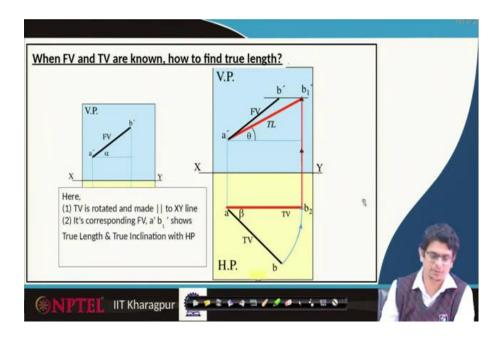
So, the angle made by this true length AB with respect to the vertical plane, that we will get it in the top view and the angle made by this true length with the horizontal we will see it on that vertical plane or in the front view. These are the directions what we will see.
