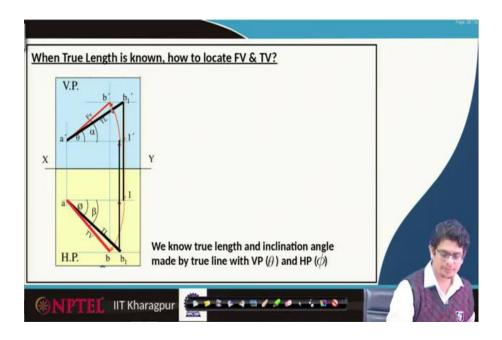
Let us ask another question when the true length is known how to locate front view and top view. So, for that purpose what we have to do, we know the true length and we know the inclination angle made by the true length with the vertical plane and also horizontal plane. This is a pretty straight forward problem, what we will do? Somehow, we already know that true length and angle made by the vertical plane, horizontal plane.
