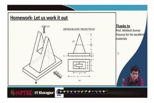
In the last class, I have asked you to construct this three-dimensional picture into projectional views. We have this kind of pin kind of structure. The answer for this pin kind of structure the views what we are going to get, this entire portion turns out to be this one, and this entire triangular one we will see it in that way. There is a dashed line at that, that portion is hidden from the backside.
