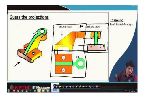
Let us look at the top view. Let us assume that is a first quadrant or first angle projection. In that, if we are looking from the top it goes to the bottom side of this front view. So, this is the front view bottom side we are supposed to draw this top view. For top view what are the things we will see?
