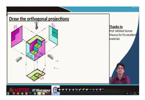
Let us look at orthogonal projections for this staircase. So, here we have a block, a rectangular block of 30 mm by 30 mm. The block perhaps fit in this box. So, if we are making something like that within that box this entire staircase construction is fixed.
