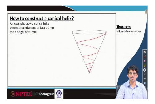
How to construct a conical helix over a cone? So, if we are winding a rope or thread around a cone sorting from apex to base, the geometric curve we get is called a conical helix. For example, let us look at a conical helix winded around a cone of base 70 mm and height 90 mm.
