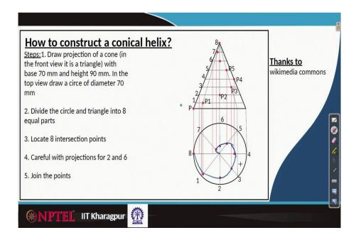
In that way, we will construct points P1, P2, P3 in the bottom view also. Then draw a line passing through these points this is the way from top view the conical helix looks like. Let us do that these steps on a graphical sheet.
