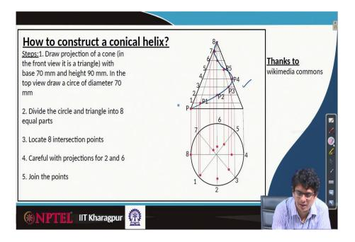
Once the stop points are made we can make a freehand sketch passing through P1, P2, P3, P4 takes a turn goes via that. This is the way we construct a conical helix winding a cone on the top side.
