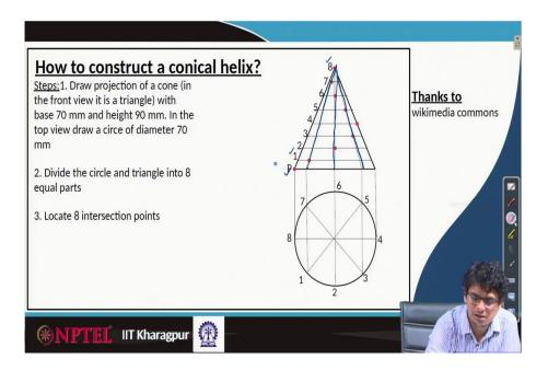
Then number them as point 1, 2, 3 to 8. Now from these labels 1, 2, 3, 4, 5, 6, 7, 8 of the circle; extend the lines which are going to generate lines on the cones. So, these are called generated lines of the cone. So, let us consider one of the particular lines.
