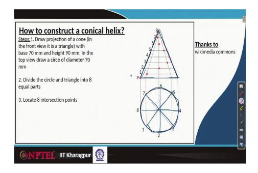
And it has made one revolution starting from the base all the way to top one. So, to do that first of all we have to construct a cone in the frontal view which we will get as a triangle. First, we have to construct a triangle of required base and height. In one of the views, if we are looking at from bottom, it looks like a circle, so one of the views is the circle we have to construct of the same diameter. Then divide the circle into 8 equal parts, number them; 1, 2, 3, 4, 5, 6, 7 and 8.
