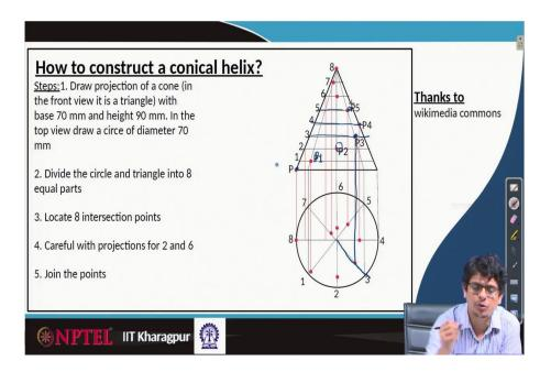
Once it is done, we will construct points or the winding rope around this cone in the frontal view. So, at this front view, we extend this 8 point going to make a point at P level similarly if we are going the intersection line of this 1 equal division and a line which is passing through 1 point that is also going to make a point P1.
