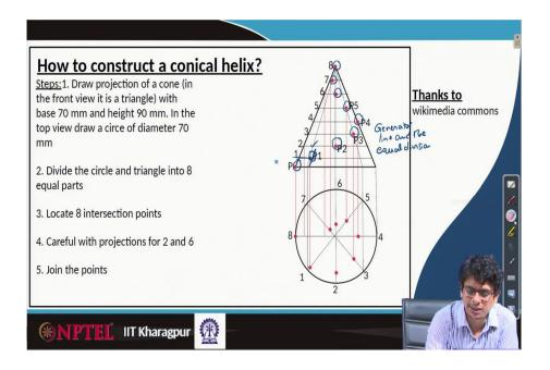
We locate points P1, 2, 3, 4, 5, 6, 7, 8. So, for the top one, we always have to intersect the generator line and the equal division made on one of the generators. So, the equal division made by one of the generators is this one intersecting with generator line 1. So, in that way, we will construct all these stop points.
