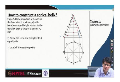
We would like to construct a generator at this point. We extend 3 lines to 5, the place where it is going to cut the base from there connect the point to peak or apex. So, this is the way we will
