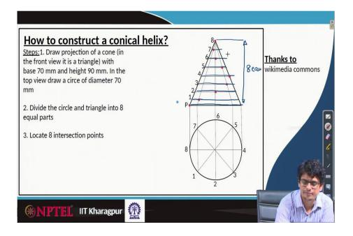
After that, divide this cone height from P to height h into 8 equal parts, this one also divides into 8 equal parts by drawing horizontal lines up to there.
