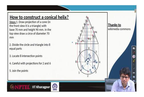
For the bottom view also, if we drop a perpendicular line from P, it is going to intersect the first line at this point locate that first point P1. Extend this P2 from one of the generator lines. Once it is done from the centre, make an arc which is going to intersect this point call it as P2, for P3 also drop a perpendicular so that it is going to intersect the 3 line call that P3, for P4 drop a line where it is intersecting call that point as P4.
