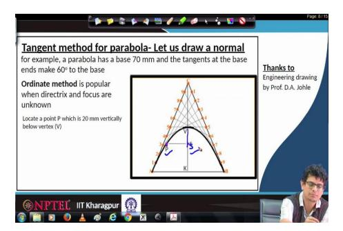
After that if we are interested in drawing a normal at a point P, let us consider this is the point P; here we would like to construct something like a normal in that direction. To do that; first of all, from vertex go below by 20 units, locate the intersection point P and on the vertical line C to K, locate another point S.
