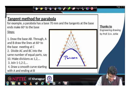
After that, join a smooth curve which passes through all these lines. So, this curve in some sense tangent to this curves, this is the way we construct a parabola by the tangent method. If we have more number of points, it will be a very smooth curve. Let us do that on the sheet. First, we have to construct six 70 mm base.
