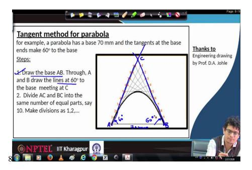
First of all, what we have to do is for a graphic construction, mark point A and B; these two points are at 70 mm apart, so this one 70 mm apart.
