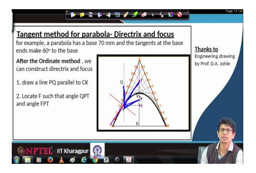
Then we have to locate focus point, focal point F such a way that,  $\angle Q P$ ,  $\angle Q P F$  is divided into two equal parts by  $\angle Q P T$  and  $\angle T P F$ ; this is the way one has to locate focus point.
