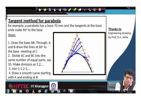
When these lines; for example, let us pick this one, 1st point and 1st point join them by a line. Similarly, 2nd point and 2nd point join them by a line; 3rd to 3rd point, similarly 6th point to 6th one let us join it.
