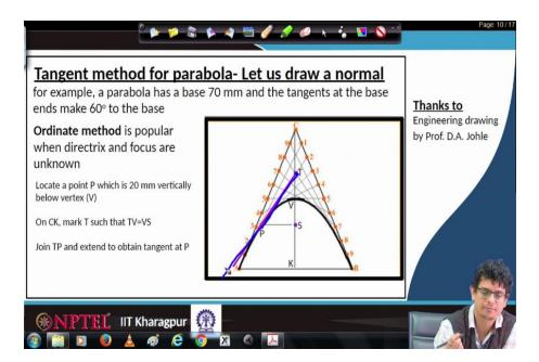
After that draw a line connecting from point T to P; if we are extending this line, this is what we call tangent line.
