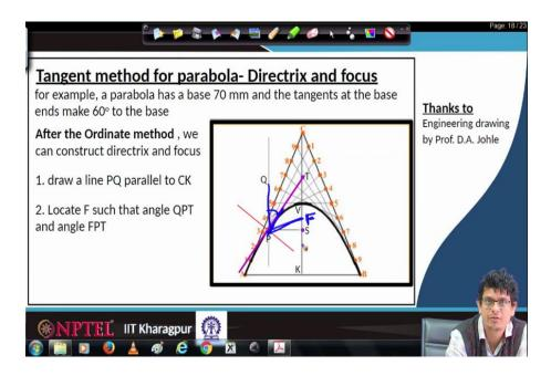
So, already we have tangent at a given chosen point, here we already constructed tangents; so first draw a vertical line, measure this angle, from that angle again reproduce another angle to focus point. If it is straight away measurable, we will be in a position to use that; otherwise angle bisector method we will use it to locate this focal point F. So, let us do that step by step.
