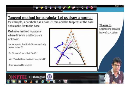
Once the tangent line is there, we can easily construct a 90 normal passing through that point; this angle supposed to be 90 and this one is a normal line, and this one is a tangent line. Let us construct that step by step.
