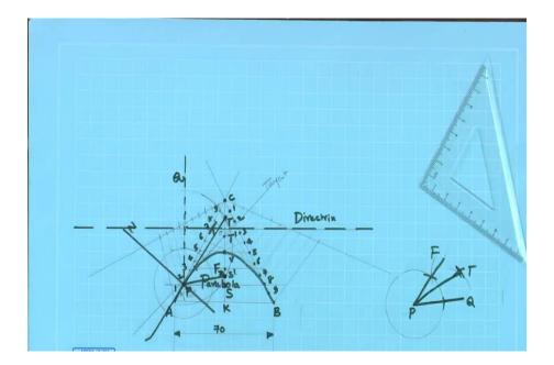
Let us draw that base on this sheet, mark 70 mm; mark these points as A and B, these are the points. After that 60 angle, we have to make with A; the tangents are making 60. Join them, A to up, so that these are going to intersect at point C.
