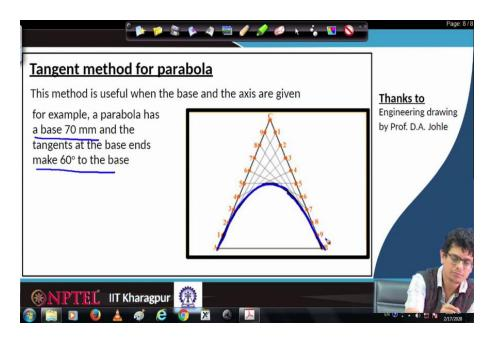
In that case, if only base 70 mm is given and tangents making 60; then how to construct a parabola which satisfies these conditions graphically?
