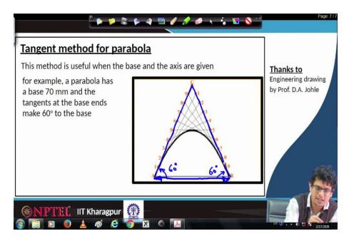
Let us look at this picture. Here the base length 70 mm is given. And the tangents; for example one of the tangent to C makes an angle 60. Similarly, the other tangent which begins at C goes all the way to B; this also makes 60.
