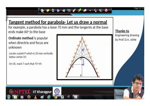
So, first of all, we have to locate P and S. After that measure the distance from V to S; from V to S whatever the distance is there, using compass from V to T also locate it. So, find this point T.
