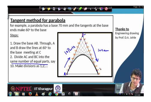
Once it is done, divide A to C into an equal number of parts, the same number of parts like 1, 2, 3 to 9; so 10 equal parts we are going to construct on this side.
