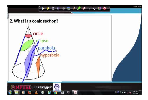
In the last classes, we have seen parabola will be constructed when a section parallel to one of the slant edges; if we are going to construct it, take a section, then we will be in a position to construct a parabola.
