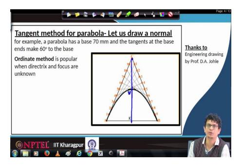
Now let us construct a normal to the drawn parabola. And this is popular as an ordinate method for constructing these normals and tangents. Further first of all what we have to do is, from C drop down a vertical line, from C to K drop a vertical line; the intersection point is the vertex of the parabola, let us name it V.
