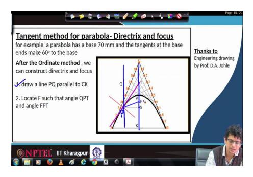
Now let us find out directrix and focus to the parabola. For this parabola construction, what we have used is, by using base and tangents, we are in a position to construct parabola. Then at any given point if we are interested in constructing parabola, tangent and normal, we went ahead measure this T V is equal to V S point and based on that we have constructed it.
