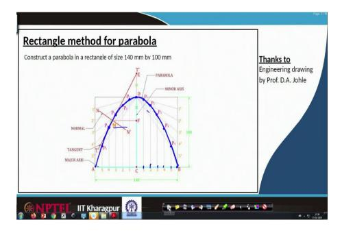
Once these points are located those are this 4 3 2 1 and D already A point is there join, these points by freehand one will be constructing this parabola. It is a symmetric one so; one can horizontally project it to get this. Otherwise, already we have constructed this 1 2 3 4 5; same procedure.
