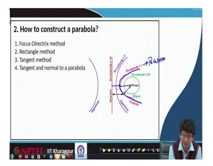
So, this is the parabola for which eccentricity is 1 that means, pick any point on parabola focus to point and directrix to that point makes equal ratio.
