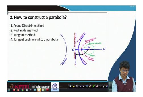
Usually, we note it by focus may be a point V on this point C on CC axis C V and V F are the same for the parabola. Further increase in eccentricity one will be going to get a hyperbola; infinite eccentricity is the vertical line or this straight line.
