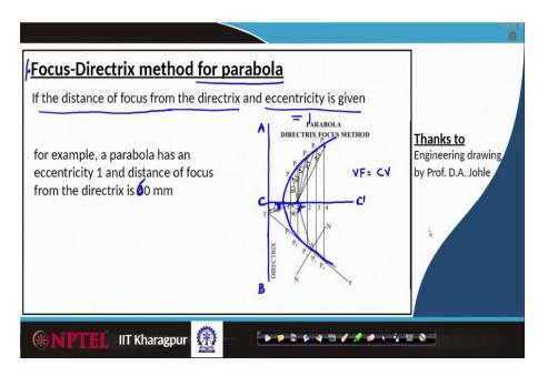
Now, using focus directrix method, the first one focus directrix method, we will construct a parabola. Suppose the distance of focus let us begin with an example. In that case, focus from the directrix is given, and eccentricity is given for parabola eccentricity always be 1, whether it is given or not.
