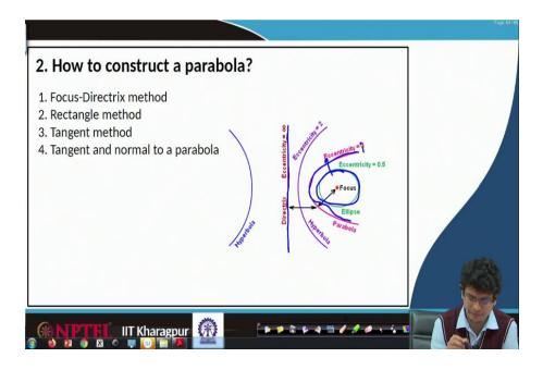
There are mainly three methods available for constructing parabola; one is using focus directrix method. The second one is the rectangle method, and the third one is the tangent method. To construct it through focus directrix method, let us recap how to construct this.
