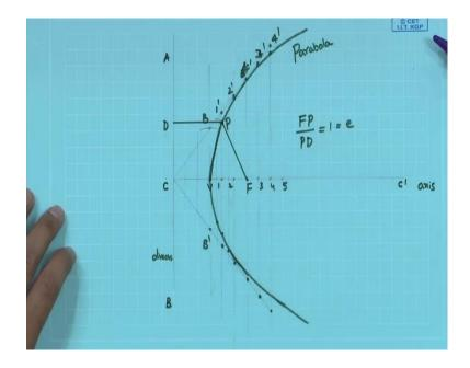
AB we have to draw first, directrix is a vertical line name it, A somewhere B draw something axis CC', which is horizontal line. Perhaps let us draw a very long line name it CC' this is axis, and this is directrix. Once it is done mark F on CC' such that CF is equal to 60 mm.
