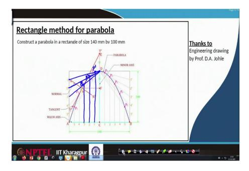
Once it is done from D point, connect the first point. Similarly from D connect the second point third point and so on. The first point the vertical projection do that, wherever it is intersecting call that point as P 1. For the second line; that means, this is the line from second point project it up intersection point P 2—similarly, the third projection on to third line P 3.
