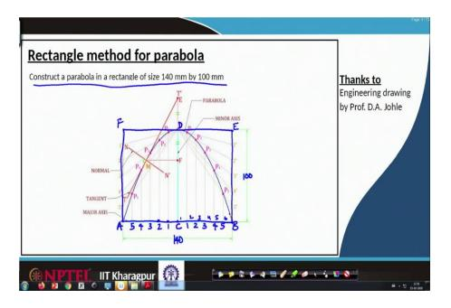
Now, we will go on to construct a second method, which is based on the rectangle method for parabola construction. In this rectangle method which we have learned for the ellipse, a similar strategy we will use. Let us look at that a parabola has to be constructed with a rectangle size of 140 mm by 100 mm. So, first of all, construct a rectangle point A point B something named D maybe E and F. So, this is 140 mm, and this is 100 mm.
