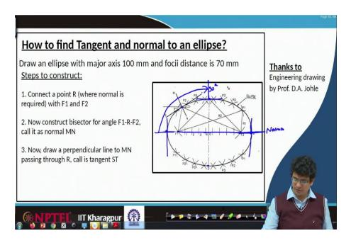
So, let us look at it carefully. If the point is straight away at the major or major axis, the procedure is to connect any point on that curve with two foci. So, if I am going to connect point B with F 1, the line will be this one. Similarly, this point we are going to connect with F 2; that means, for this point B again connect that. Both are still making that  $0^{\circ}$  or  $180^{\circ}$  kind of thing the equal division which comprises of the same line.
