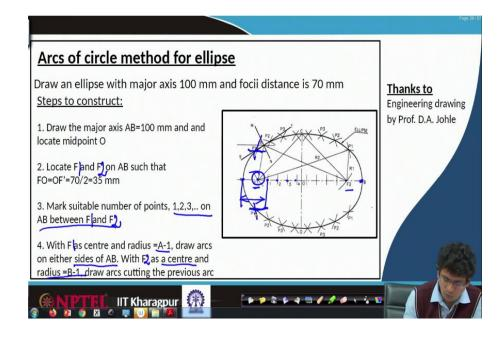
Now, we have to mark the suitable number of points something like 1, 2, 3, on AB between F 1 and F 2. F 1 and F 2 it can be equal or any number of points. It is easy always to go with an equal number of points as a uniform grid first point, second point, third point, fourth point.
