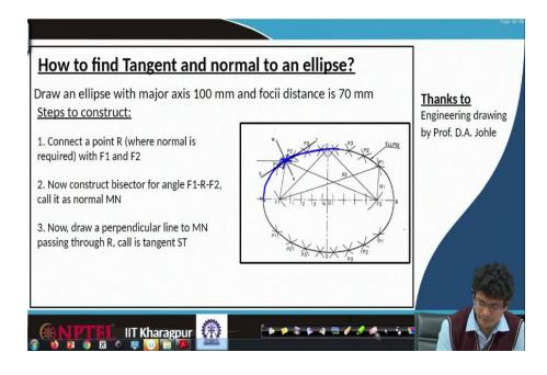
Now, we will ask a question: how to draw a tangent and normal to an ellipse. For example, part of the curve we have constructed as an ellipse. Now, pick any point where we would like to construct a normal or tangent. In this case, we would like to construct, for example, at point R. So, this is the ellipse which we have joined, and we intend to construct something like normal to that. For that purpose, what we have to do?
