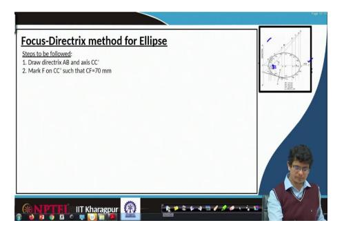
So, somewhere at point C draw a line name it CC'. Once it is done mark a point F on CC'. So, we have already constructed AB and CC'. So, now locate a focus F, which will be at 70 mm.
