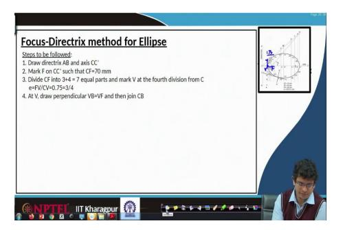
So, we have already located point V on that curve. So, there using a mini drafter draw a perpendicular line this is the one. So this point is V somewhere point B, such that V B is equal to V F. So, V we know F we know on that perpendicular line what is this distance V F equal distance move it name it as B.
