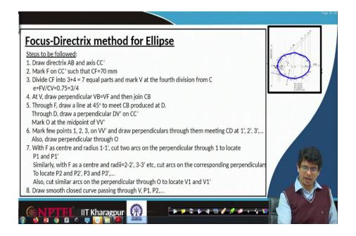
So, once we are done with this entire procedure, a smooth curve passing through this V point P 1 P 2 P 4 and so on, we will be in a position to construct an ellipse.
