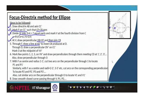
So, the 1st point draw directrix AB and CC' we have noted down, then mark F on CC'. Second step is we have to mark CC' such that C F is equal to 70 mm C is this point F is that point.
