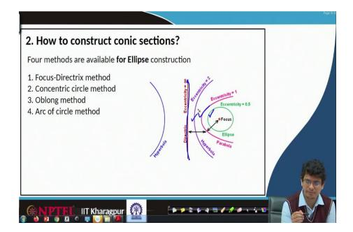
Furthermore, there is a line which we call directrix line, about this directrix line one will be in a position to construct an ellipse parabola or a hyperbola.
