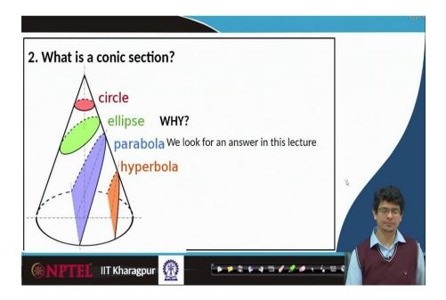
If a parallel slant cut section if we are taking it to construct a hyperbola and any other section it makes hyperbola.
