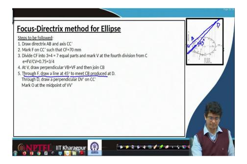
So, already we have noted C point and B point this we have extended, then from F a  $45^{\circ}$  line we have to construct it extends down to meet tangent, so this angle is  $45^{\circ}$ s. So, that we have an intersection point let us call that point as D.
