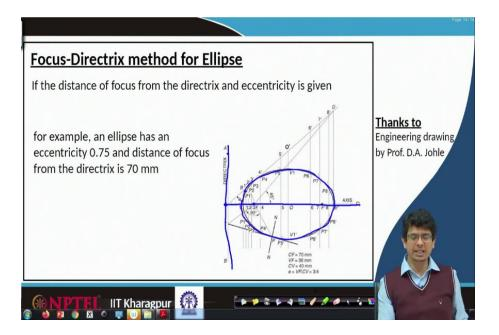
So, using this directrix focus method, first of all, we will be drawing this directrix. We will be going to construct something like a line C from directrix to that focal point we will locate it something like 70 mm, do geometric construction then draw tangent lines and vertical lines horizontal lines construct intersecting points, then follow the procedure to fill this gap like an ellipse. We will see that step by step.
