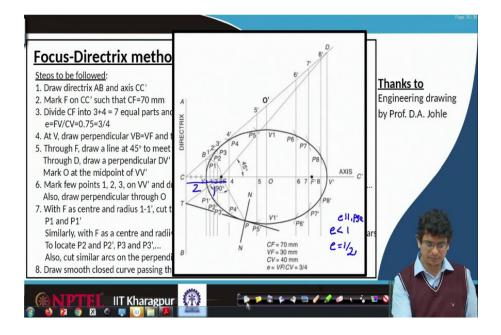
If it is something like another factor any e less than 1 we get an ellipse, in this case, we have used three fourth; one can also use something like half. If e is equal to half three fourth ratio 0.75, it makes. So, 1 2 ratio means that we have to make it into 3 parts first of all, then locate 2 parts in that direction 1 part then go with the same procedure we will get another ellipse. This is the way any general ellipse one will be in a portion to construct it.
