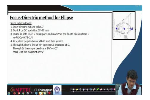
So, V is one end another end for this ellipse is VV'. We know perpendicular bisector how to draw that. So, using VV' use arcs construct then drop it. So, that perpendicular bisector O we will be in a portion to know. Then mark a few points 1, 2, 3 on VB'.
