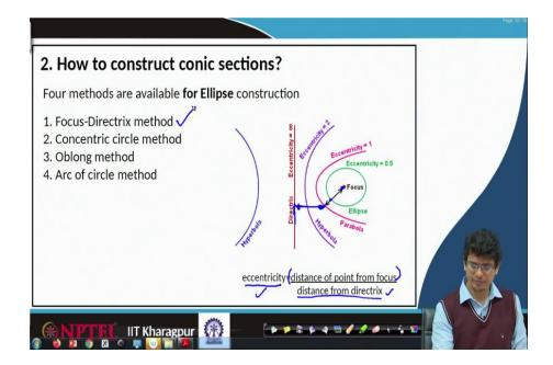
Furthermore, we call that ratio as eccentricity. So, eccentricity is defined as the distance of a point from the focus. For example, if it is an ellipse this point to that point. If it is a parabola from this point to that point distance of that point from there to focus by distance from directrix for that point.
