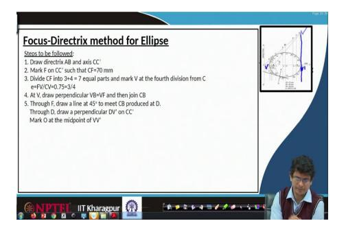
Now, through D, draw perpendicular lines D V' on C. So, this is the intersection point So, use your mini drafter construct a vertical line perpendicular thing thus name it V', on one side we have V, on another side we have V'.
