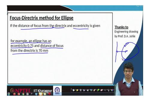
So, a directrix and perhaps an arbitrary curve it has a focus So, distance from directrix will be given to the focus and what kind of eccentricity, whether it is lower than 1 greater than 1 will be given if that is the case construct this arbitrary curve. For example, here an ellipse has an eccentricity 0.75, any eccentricity less than 1 we will be getting this ellipse and distance of focus from the directrix is 70 mm, if that is the case construct an ellipse.
