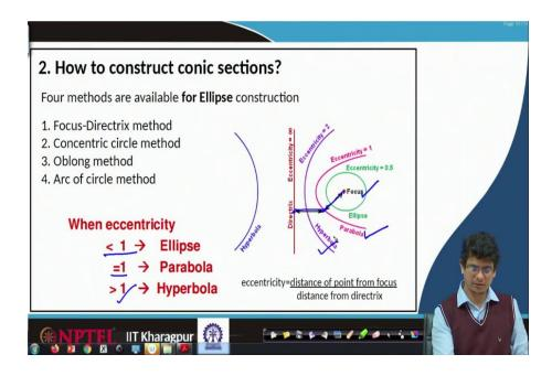
If the eccentricity is less than 1 we get an ellipse, if it is equal to 1, we get a parabola, that means from focus to point on this parabola and distance from this point to this directrix they are the same. Because the ratio is 1, such kind of curve what we call parabola, if that eccentricity is greater than 1, we get a hyperbola.
