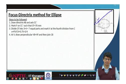
Then join B point to C point. So, once we locate that point join it. We have already this F point focus draw the line at 45°s. So, through F point, draw the line at 45°s to meet CB.
