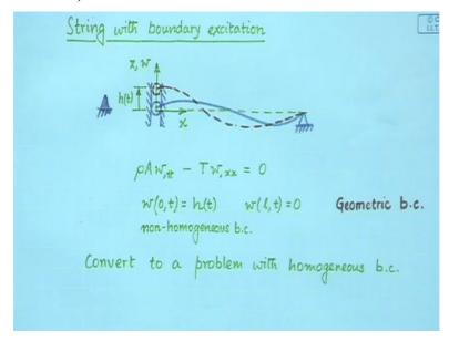
Now let us look at an example of a string with boundary excitation. So we will put a string which is free to slide on this left boundary. I will draw a displaced configuration of the strain. So we will assume that this string is being driven by a robust actuator which actually gives a displacement condition on the boundary. So this string is being excited by a system or an actuator which is robustly driving the left boundary.
