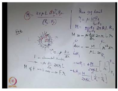
Let us say we have concentric cylinders and the speciality of this system is that maybe one of the cylinders is having a relative motion with respect to the other. So let us take an example where the outer cylinder is stationary, outer one is stationary and the inner wall is rotating with a particular angular speed omega. There is a fluid that is present in the gap between the 2 cylinders.
