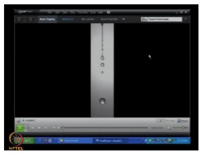
And the third example. This is like a train of droplets and you see the droplets are like, these are not like rigid spheres. So they are continuously deforming and you see the way in which these droplets are moving. So initially one big droplet and then you see that there are trains of droplets of different sizes and they are continuously interacting with each other. So at least you can appreciate that this is beautiful.
