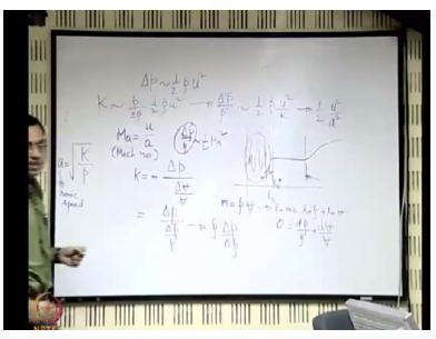
So in the numerator you have u, in the denominator you have a. So u is the velocity of flow and a is the velocity of a disturbance which is moving in the medium in which the flow is occurring and these 2 ratios is known as Mach number, I mean, ratios of these 2 numbers is known as Mach number. So you have heard about the Mach number like a jet moving with a Mach of this. So to have the Mach number, here is the velocity of flow relative to the velocity of the
