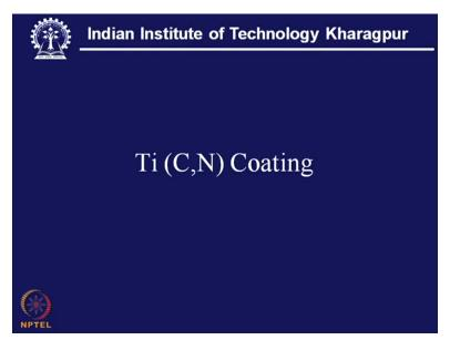
So this is TiCN coating. Because titanium carbide is well known since the cutting tool came into being and also titanium nitride it is known for its chemical stability, so it is titanium carbo-nitride coating which can have also well strategic application. And some of those strategic areas, carbo-nitride coating can be found out to be one of the very best candidate.
